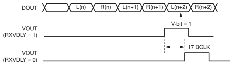
Figure 8. RXVDLY and VOUT Timing
