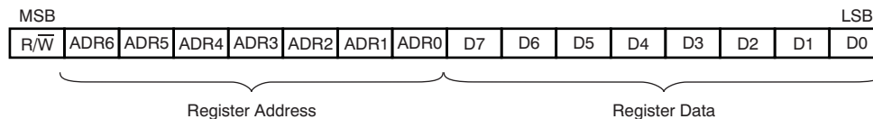
Figure 19. Control Data Word Format for MDI
