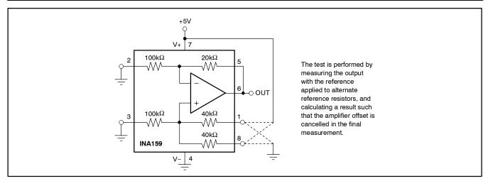
Figure 2. Test Circuit for Reference Divider Accuracy
