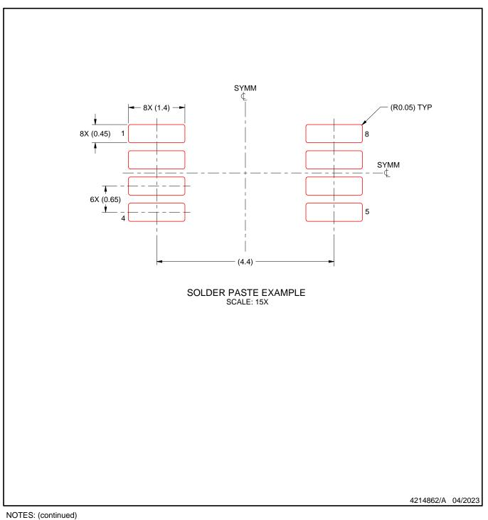
11. Laser cutting apertures with trapezoidal walls and rounded corners may offer better paste release. IPC-7525 may have alternate design recommendations.
