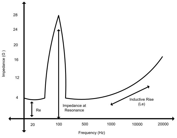
Figure 7-11. Speaker Impedance Measurement
