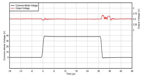
Figure 6-4. Enhanced PWM Rejection Performance
