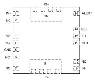
Figure 4-1. INA790x DEK Package 15-Pin VQFN Top View
