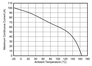
Figure 6-2. Maximum Continuous Current vs Ambient Temperature
