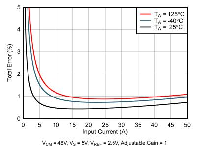
Figure 7-1. INA790A Total Error vs Input Current
