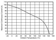
Maximum Continuous Current vs Ambient Temperature
