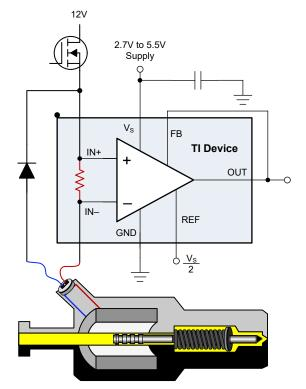
Figure 7-8. Solenoid Drive Application Circuit
