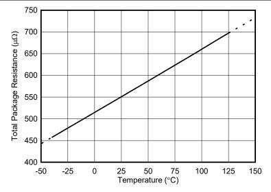
Figure 6-1. IS+ to IS– Package Resistance vs Temperature
