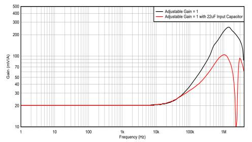
Figure 7-4. INA790x Gain vs Frequency Before and After Adding 22µF Input Capacitor
