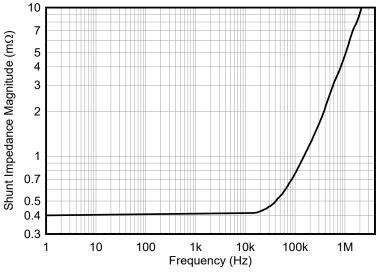
Figure 7-3. Shunt Impedance vs Frequency
