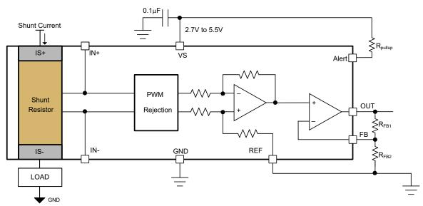
Figure 6-6. Ground-Referenced Output
