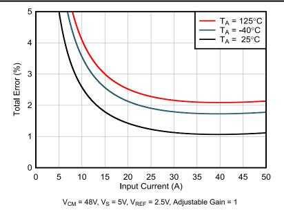
Figure 7-2. INA790B Total Error vs Input Current
