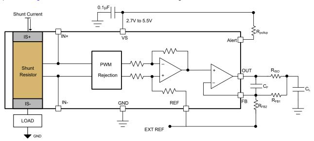
Figure 7-5. INA790x With RISO-Dual-Feedback
