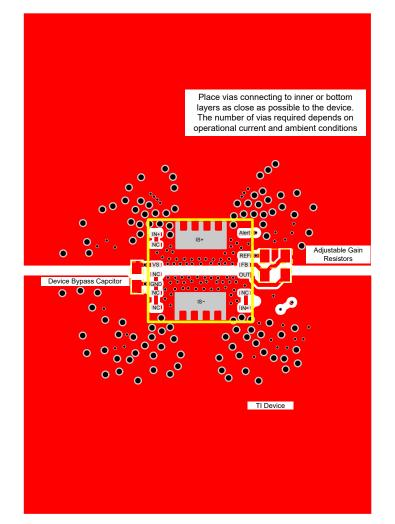
Figure 7-12. INA790x Layout Example
