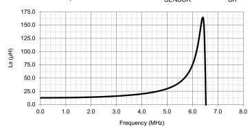
Figure 54. Example Coil Inductance vs. Frequency
