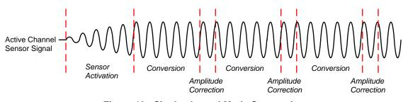
Figure 13. Single-channel Mode Sequencing
