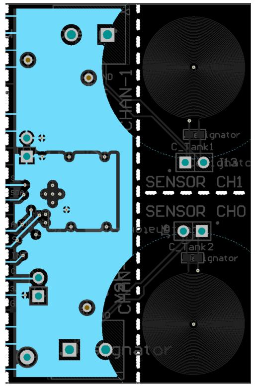
Figure 59. Example PCB Layout: Mid-layer 2 (Power)
