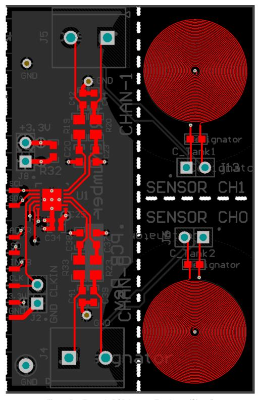
Figure 57. Example PCB Layout: Top Layer (Signal)
