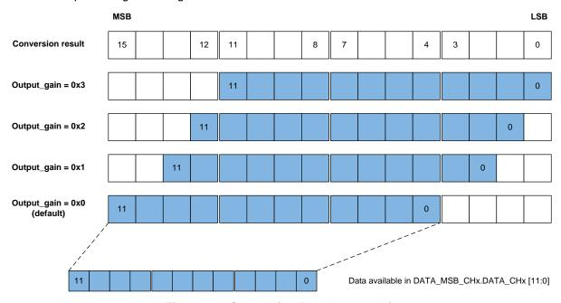
Figure 14. Conversion Data Output Gain
