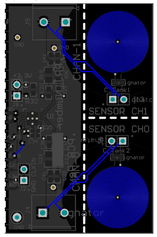
Figure 60. Example PCB Layout: Bottom Layer (Signal)
