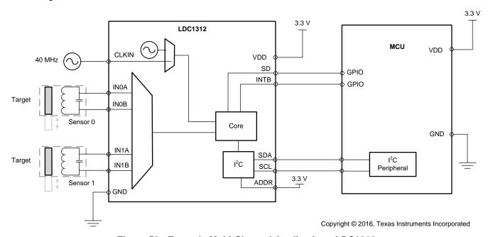
Figure 53. Example Multi-Channel Application - LDC1312
