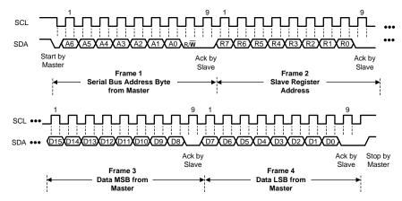
Figure 15. I2C Write Register Sequence
