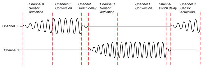
Figure 12. Multi-channel Mode Sequencing
