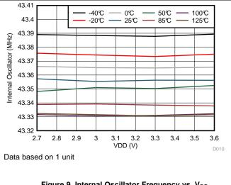
Figure 9. Internal Oscillator Frequency vs. V<sub>DD</sub>
