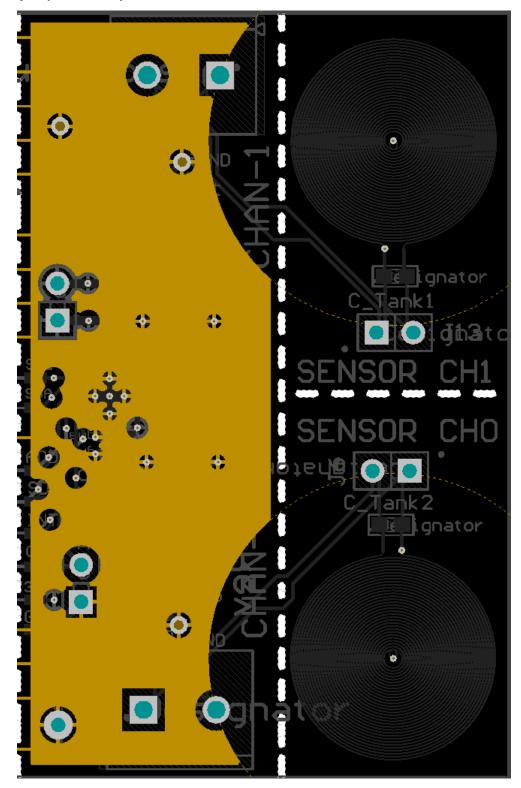
Figure 58. Example PCB Layout: Mid-layer 1 (GND)
