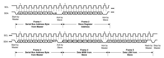
Figure 16. I2C Read Register Sequence
