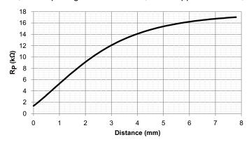
Figure 51. Example RP vs. Distance with a 14-mm PCB Coil and 2mm Thick Stainless Steel Target
