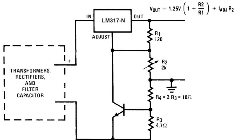
—Short circuit current is approximately  $\frac{600\text{ mV}}{R_3}$ , or 210 mA
