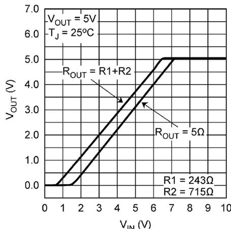
Figure 19.  $V_{OUT}$  vs  $V_{IN}$ ,  $V_{OUT} = 5V$
