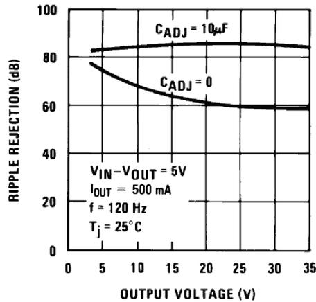
Figure 9. Ripple Rejection
