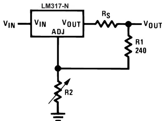
**Figure 16. Regulator With Line Resistance in Output Lead**
