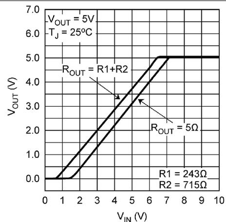
Figure 6.  $V_{OUT}$  vs  $V_{IN}$ ,  $V_{OUT} = 5V$
