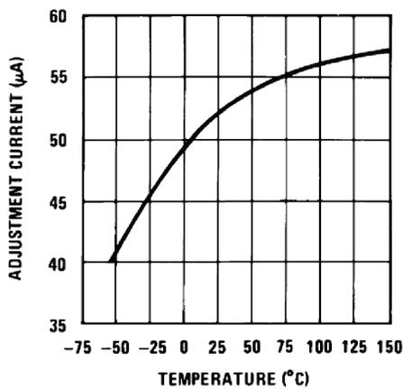
Figure 3. Adjustment Current
