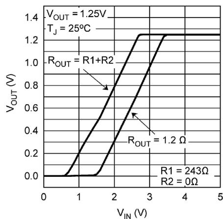
Figure 5.  $V_{OUT}$  vs  $V_{IN}$ ,  $V_{OUT} = V_{REF}$
