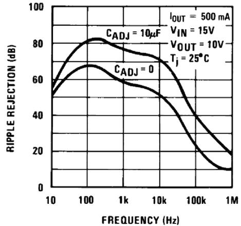
Figure 10. Ripple Rejection
