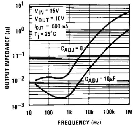
Figure 12. Output Impedance
