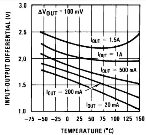
Figure 4. Dropout Voltage
