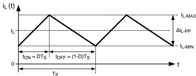
**Figure 12. Ideal CCM Regulator Inductor Current  $i_L(t)$**
