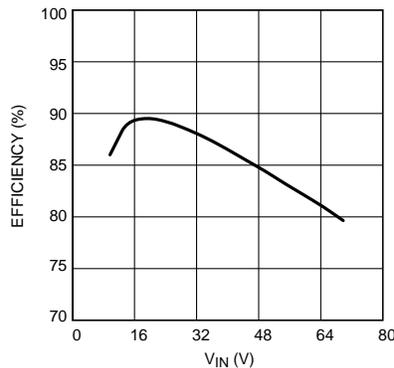
**Figure 30. Buck-Boost Efficiency vs Input Voltage, V<sub>O</sub>= 6 LEDs**
