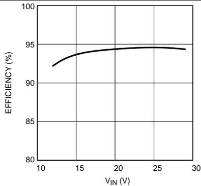
**Figure 1. Boost Efficiency vs Input Voltage**
