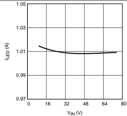
**Figure 4. Buck-boost LED Current vs Input Voltage**
