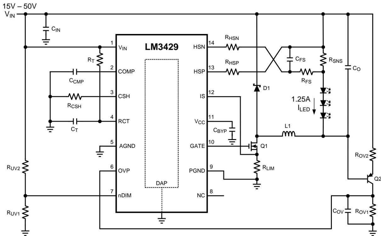
**Figure 35. Buck Application - 3 LEDs at 1.25 A Schematic**
