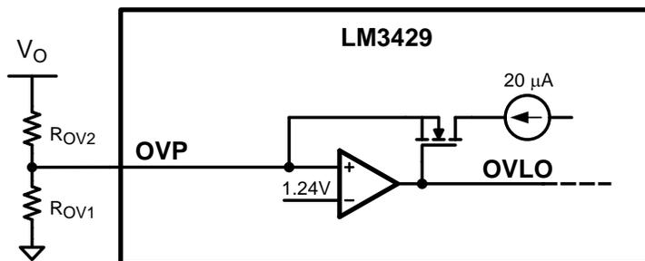
Figure 21. Overvoltage Protection Circuitry
