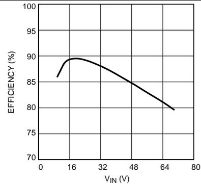
**Figure 2. Buck-Boost Efficiency vs Input Voltage**
