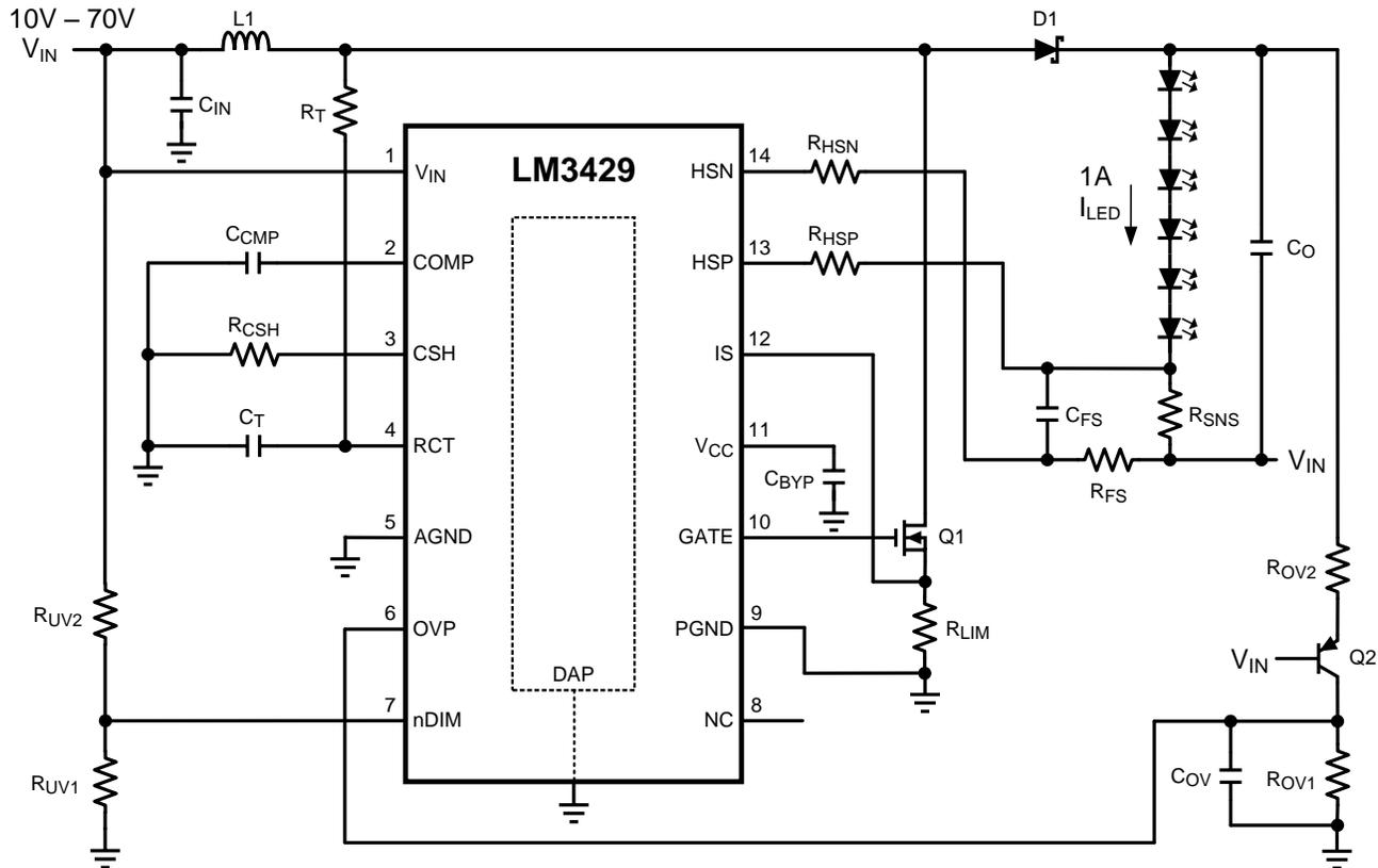
**Figure 29. Buck-Boost Application - 6 LEDs at 1 A Schematic**
