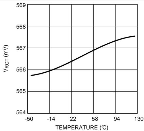
**Figure 9.  $V_{RCT}$  vs. Junction Temperature**
