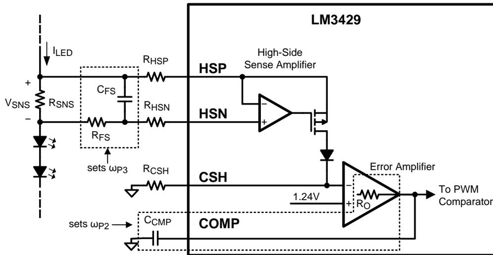
Figure 19. Compensation Circuitry
