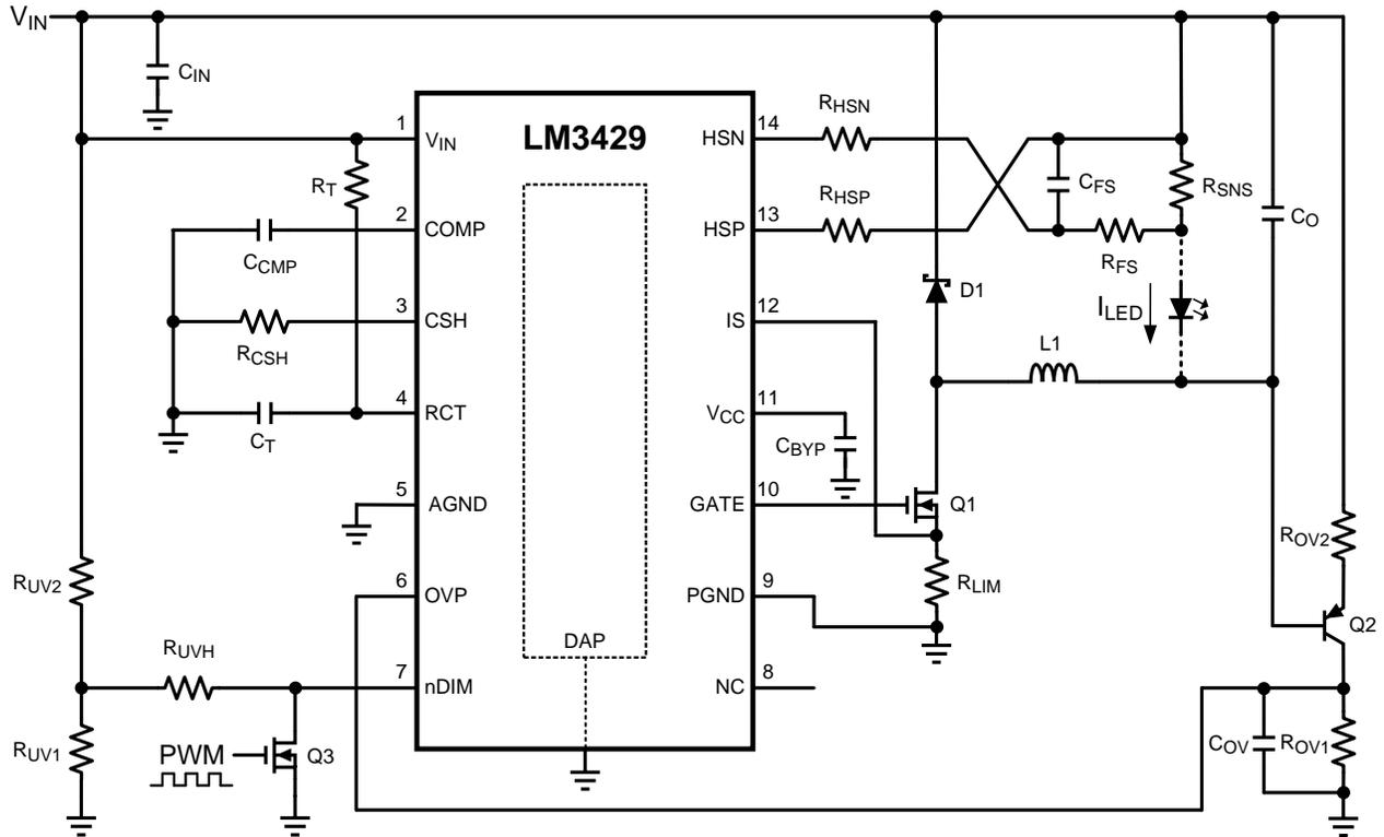
Figure 27. Buck Regulator ( $V_{IN} > V_O$ )
