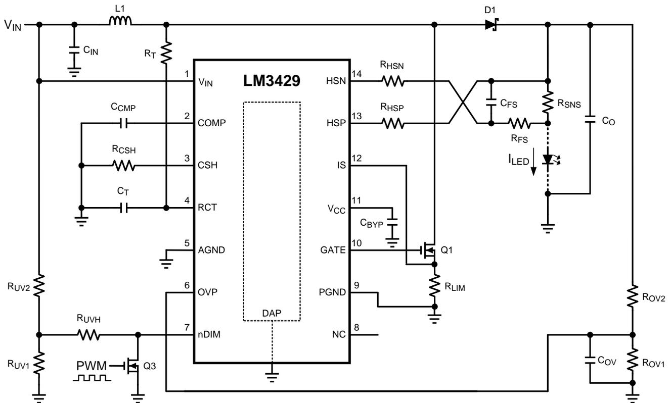
**Figure 26. Boost Regulator ( $V_{IN} < V_O$ )**
