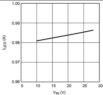
**Figure 3. Boost LED Current vs Input Voltage**
