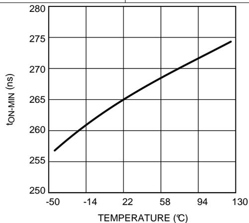
**Figure 11.  $t_{ON-MIN}$  vs. Junction Temperature**
