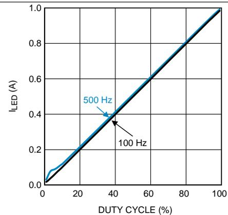
**Figure 6. PWM Dimming**
