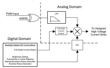
Figure 14. PWM Input Architecture
