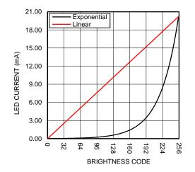
Figure 19. LED Current Mapping Modes
