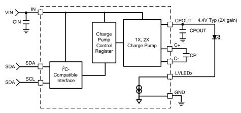
Figure 18. Integrated Charge Pump
