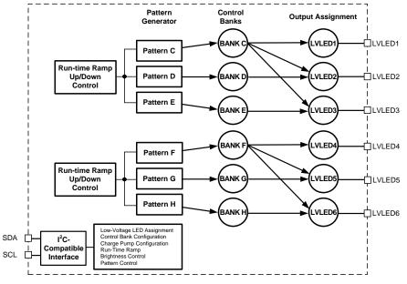
Figure 17. Low-Voltage LED Functional Control Diagram
