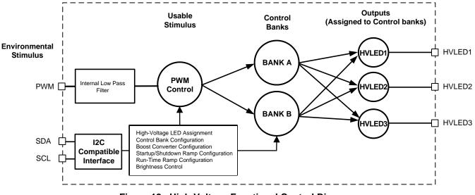
Figure 12. High-Voltage Functional Control Diagram
