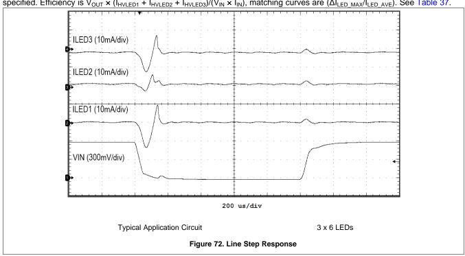
$V_{IN} = 3.6 \text{ V}, V_{LED} = 3.2 \text{ V} @ 20 \text{ mA}, \text{Typical Application Circuit}, T_A = 25^{\circ}\text{C}, \text{Full-Scale Current} = 20.2 \text{ mA} \text{ unless otherwise}$ specified. Efficiency is  $V_{OUT} \times (I_{HVLED1} + I_{HVLED2} + I_{HVLED3})/(V_{IN} \times I_{IN})$ , matching curves are  $(\Delta I_{LED\_MAX}/I_{LED\_AVE})$ . See Table 37.
