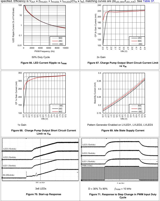
$V_{IN} = 3.6 \text{ V}, V_{LED} = 3.2 \text{ V} @ 20 \text{ mA}$ , Typical Application Circuit,  $T_A = 25^{\circ}\text{C}$ , Full-Scale Current = 20.2 mA unless otherwise specified. Efficiency is  $V_{OUT} \times (I_{HVLED1} + I_{HVLED2} + I_{HVLED3})/(V_{IN} \times I_{IN})$ , matching curves are ( $\Delta I_{LED_MAX}/I_{LED_AVE}$ ). See Table 37.
