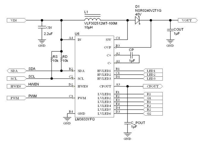
Figure 23. LM3633 Simplified Schematic
