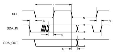
Figure 1. I<sup>2</sup>C-Compatible Interface Timing
