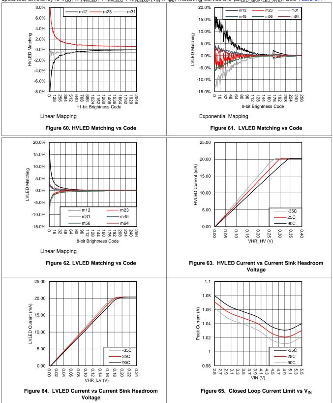
$V_{IN} = 3.6 \text{ V}, V_{LED} = 3.2 \text{ V} @ 20 \text{ mA}$ , Typical Application Circuit,  $T_A = 25^{\circ}\text{C}$ , Full-Scale Current = 20.2 mA unless otherwise specified. Efficiency is  $V_{OUT} \times (I_{HVLED1} + I_{HVLED2} + I_{HVLED3})/(V_{IN} \times I_{IN})$ , matching curves are ( $\Delta I_{LED_MAX}/I_{LED_AVE}$ ). See Table 37.
