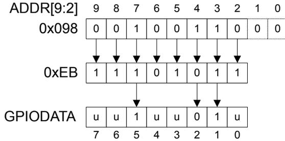
During a read, if the address bit associated with the data bit is set to 1, the value is read. If the address bit associated with the data bit is set to 0, it is read as a zero, regardless of its actual value. For example, reading address **GPIODATA** + 0x0C4 yields as shown in Figure 8-3 on page 294.
