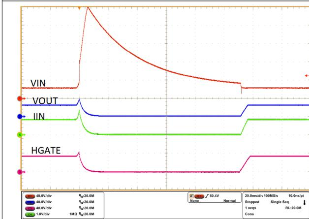
**Figure 8-4. Unsuppressed Load Dump 200 V - Output Cut-off**
