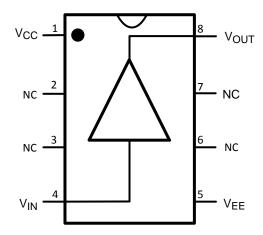
Figure 2. 8-Pin SOIC (Top View) See Package Number D (R-PDSO-G8)
