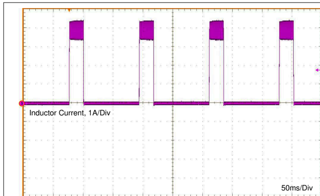
Figure 8-5. Inductor Current Burst in Short-Circuit Mode
