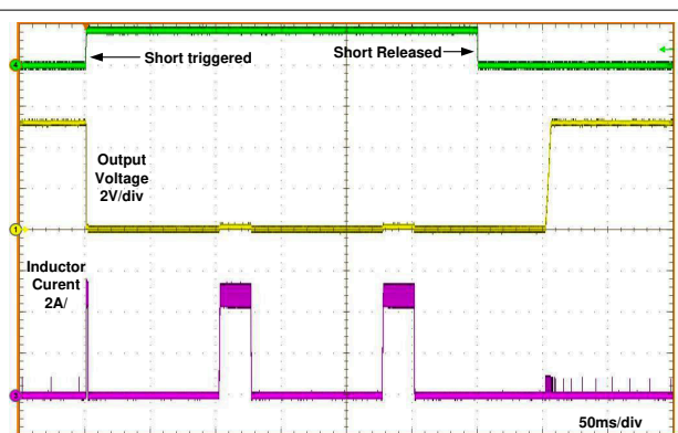
Figure 8-6. Short-Circuit Transient and Recovery V_{IN} = 12\text{ V} , V_{OUT} = 5\text{ V}
