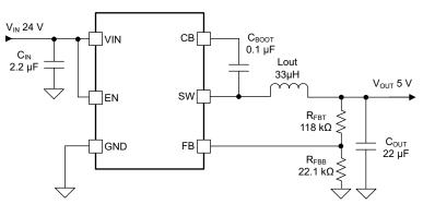
Figure 8-1. Application Circuit
