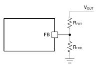
Figure 7-2. Output Voltage Setting
