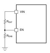
Figure 7-3. System UVLO by Enable Divider
