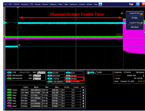
Figure 5-19. Channel Enable Setting Time
