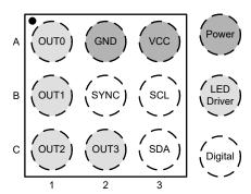
Figure 5-1. LP5810 YBH Package 9-Pin DSBGA Top View
