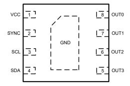
Figure 5-2. LP5810 DSD Package 8-Pin WSON Top View
