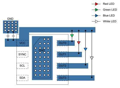
Figure 9-6. LP5810 WSON Package Layout Example
