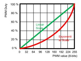
Figure 7-3. Linear and Exponential PWM Dimming Curves
