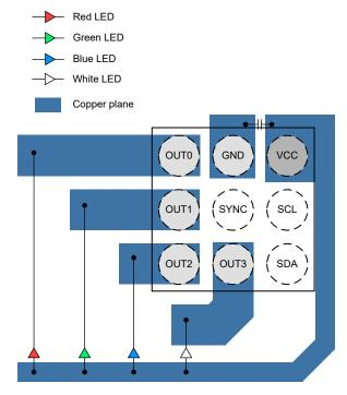
Figure 9-5. LP5810 DSBGA Package Layout Example
