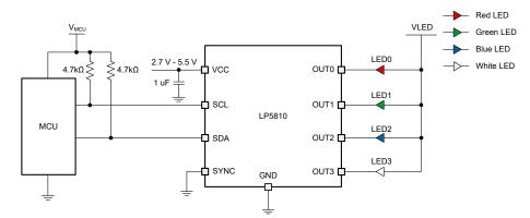
Figure 9-1. Typical Application - LP5810 Driving RGBW LEDs
