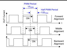
Figure 7-2. PWM Alignment Scheme
