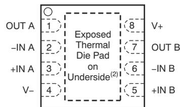
**Figure 4-4. OPA2328 DRG Package, 8-Pin WSON (Top View)**
