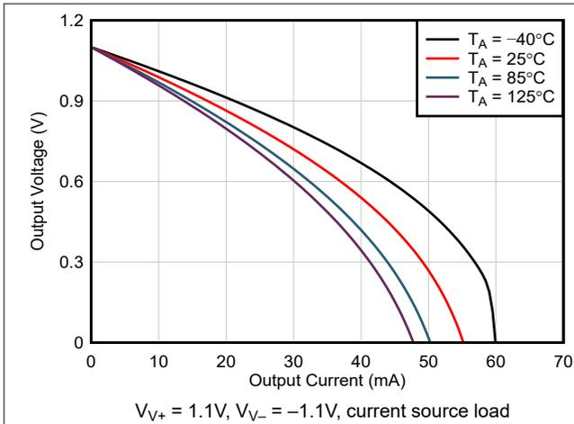
**Figure 5-19. Output Voltage Swing vs Output Current**
