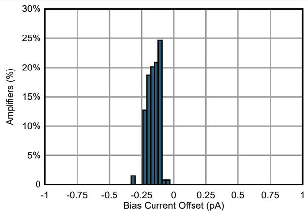
Figure 5-12. Input Bias Offset Current Distribution
