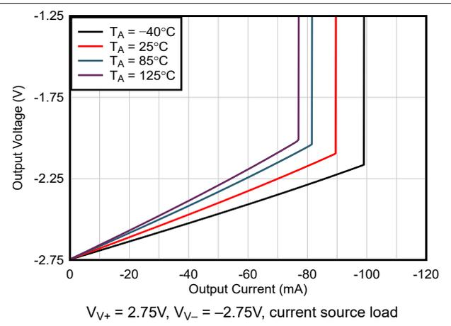
**Figure 5-22. Output Voltage Swing vs Output Current**
