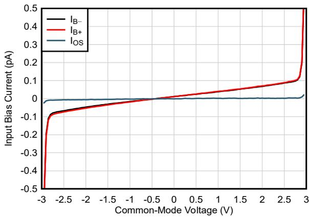
Figure 5-7. Input Bias Current vs Common-Mode Voltage
