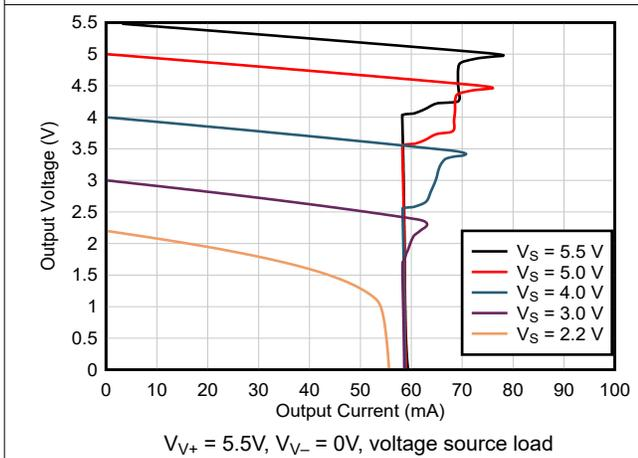
**Figure 5-23. Output Voltage Swing vs Output Current**
