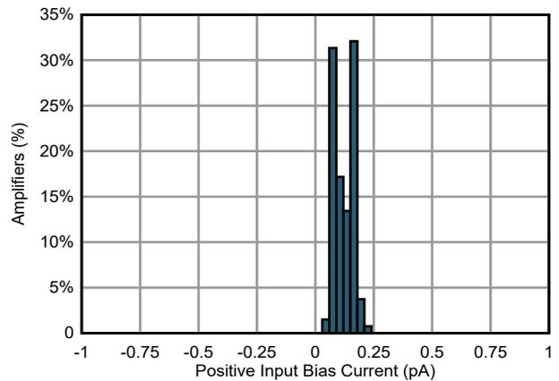
Figure 5-10. Positive Input Bias Current Distribution
