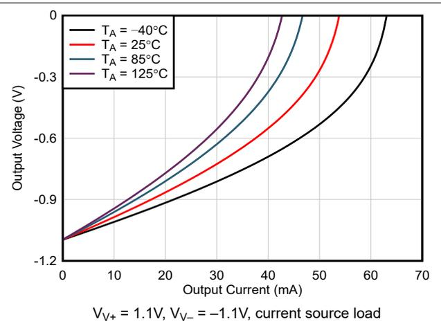
**Figure 5-20. Output Voltage Swing vs Output Current**
