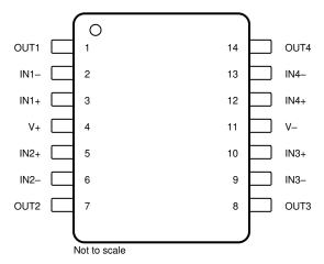
Figure 5-1. OPA4991-EP DYY Package 14-Pin SOT-23 (Top View)
