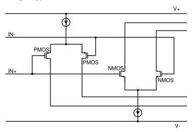
Figure 7-8. Rail-to-Rail Input Stage
