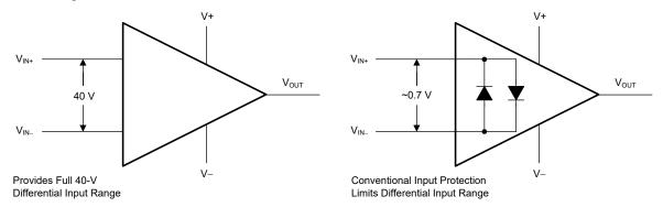
Figure 7-1. OPA4991-EP Input Protection Does Not Limit Differential Input Capability
