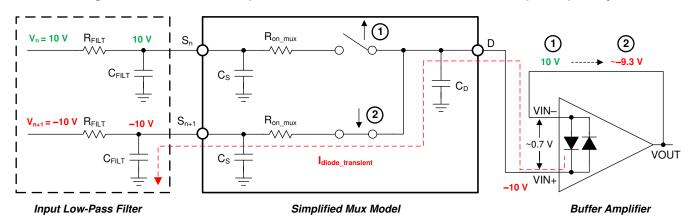
Figure 7-2. Back-to-Back Diodes Create Settling Issues
