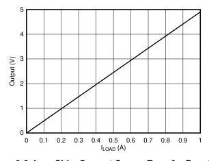
Figure 8-2. Low-Side, Current-Sense, Transfer Function
