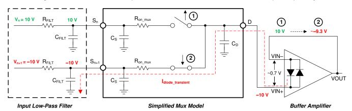
Figure 7-2. Back-to-Back Diodes Create Settling Issues
