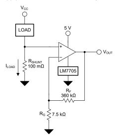
Figure 8-1. OPA4H199-SEP in a Low-Side, Current-Sensing Application
