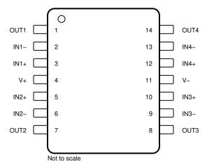
Figure 5-1. OPA4H199-SEP DYY Package 14-Pin SOT-23 (14) Top View
