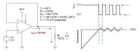
Figure 7-4. Thermal Protection
