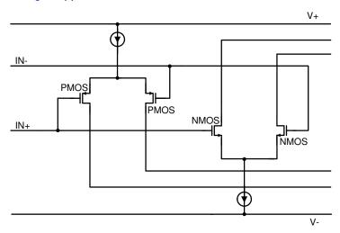
Figure 7-8. Rail-to-Rail Input Stage
