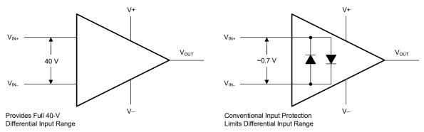
Figure 7-1. OPA4H199-SEP Input Protection Does Not Limit Differential Input Capability
