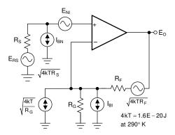
Figure 8-10. Operational Amplifier Noise Analysis Model
