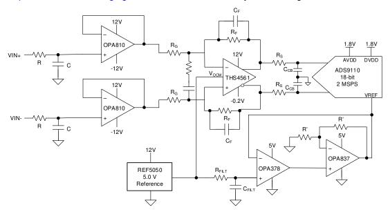
Figure 8-15. High-Z Input Data Acquisition Front-End
