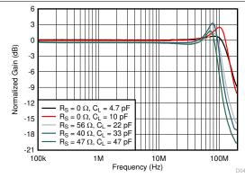
See Figure 8-1 and Figure 7-1,  $V_O = 20 \ mV_{PP}, \ gain = 1 \ V/V, \ R_F = 0 \ \Omega$
