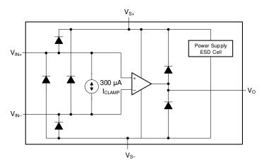
Figure 7-2. Internal ESD Protection
