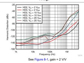
Figure 6-22. Harmonic Distortion vs Frequency vs Vo
