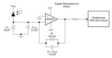
Figure 8-12. Wideband, High-Sensitivity, Transimpedance Amplifier
