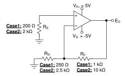
Figure 8-11. Comparing Noise Contributors for Two Cases with the Amplifier in a Noninverting Gain of  $5\,\text{V/V}$
