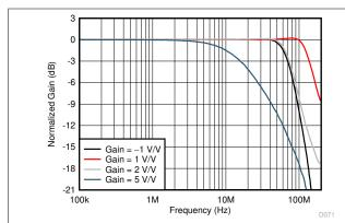
See Figure 8-1 and Figure 8-2,  $V_O = 20 \text{ mV}_{PP}$
