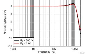
See Figure 8-1,  $V_O$  = 20 m $V_{PP}$ , gain = 1 V/V,  $R_F$  = 0  $\Omega$
