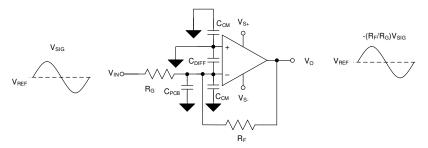
Figure 8-5. Inverting Amplifier With Input Capacitors
