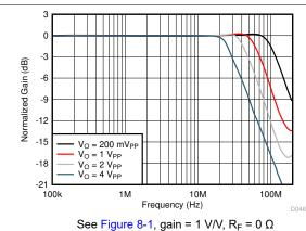
Figure 6-5. Large-Signal Frequency Response vs Output Voltage
