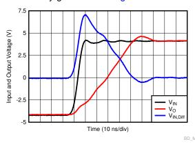
Figure 8-18. Large-Signal Transient Response Using the OPA810
