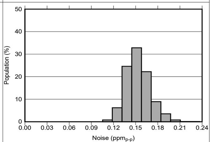
Figure 6-6. 0.1Hz to 10Hz Voltage Noise Distribution
