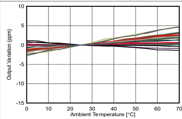
Figure 6-1. Output Voltage Vs Free-Air Temperature
