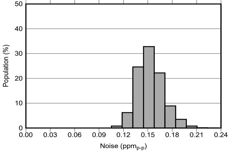
**Figure 8-5. 0.1Hz to 10Hz Voltage Noise Distribution**
