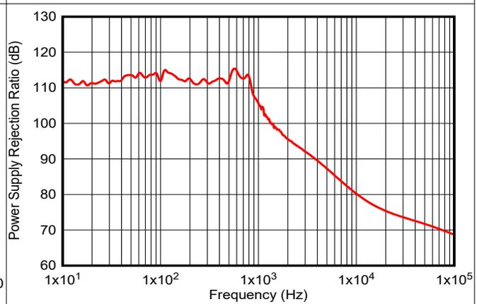
Figure 6-10. Power-Supply Rejection Ratio vs Frequency
