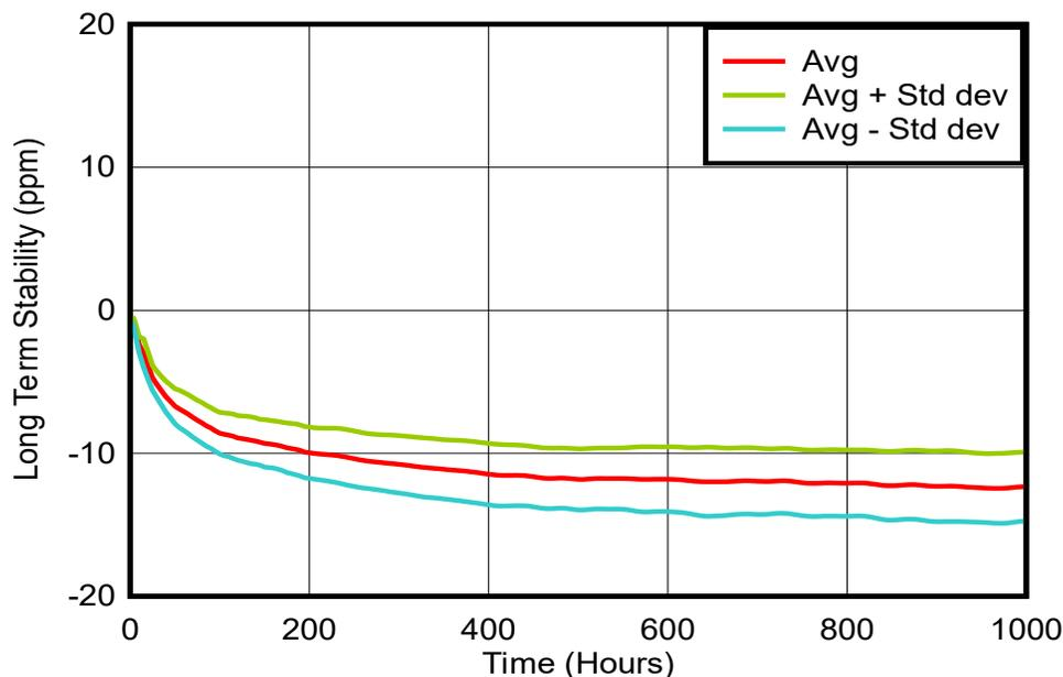
Figure 8-1. Long Term Stability ( $V_{REF\_Z}$ )
