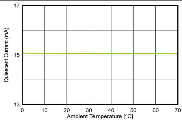
Figure 6-4. Supply Current ( $I_{VDD}$ ) vs Temperature
