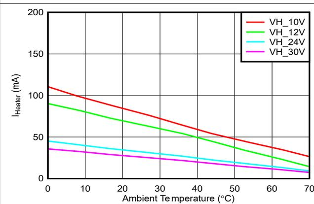
Figure 6-5. Heater Current ( $I_{Heater}$ ) vs Temperature
