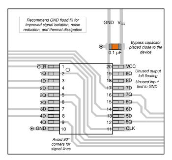
Figure 8-3. Layout Diagram
