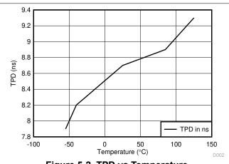
Figure 5-2. TPD vs Temperature
