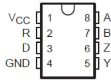
**Figure 4-1. D or P Package (Top View)**
