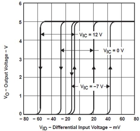
**Figure 5-8. Receiver Output Voltage vs Differential Input Voltage**
