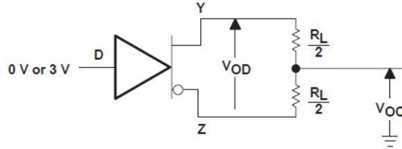
Figure 6-1. Differential and Common-Mode Output Voltage Test Circuit
