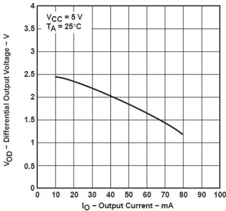
Figure 5-3. Driver Differential Output Voltage vs Output Current
