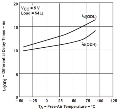
Figure 5-5. Driver Differential Delay Time vs Free-Air Temperature
