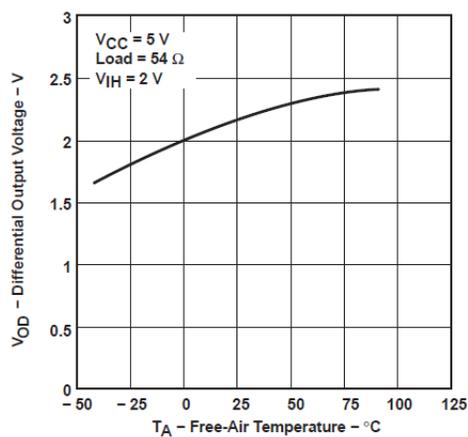
Figure 5-4. Driver Differential Output Voltage vs Free-Air Temperature
