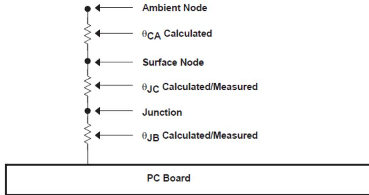
Figure 7-2. Thermal Resistance
