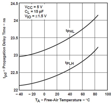
**Figure 5-11. Receiver Propagation Delay Time vs Free-Air Temperature**
