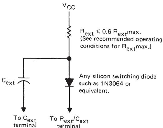
TIMING COMPONENT CONNECTIONS WHEN
