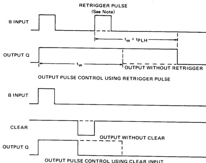
NOTE: Retrigger pulses starting before  $0.22 C_{ext}$  (in picoseconds) nanoseconds after the initial trigger pulse will be ignored and the output duration will remain unchanged.
