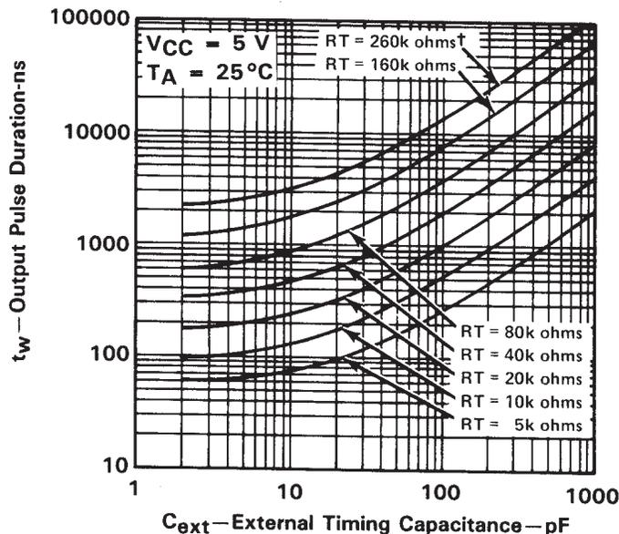
† This value of resistance exceeds the maximum recommended for use over the full temperature range of the SN54LS circuits.
