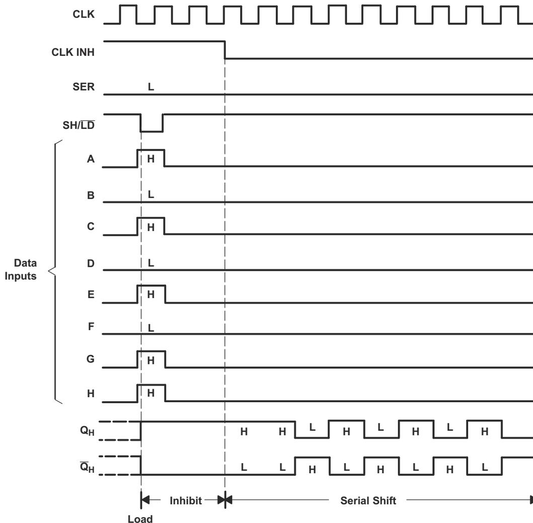
Figure 6-1. Typical Shift, Load, and Inhibit Sequences
