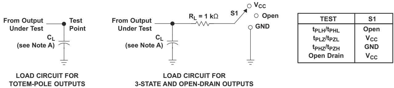
LOAD CIRCUIT FOR TOTEM-POLE OUTPUTS
