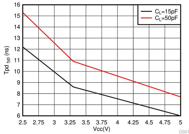
Figure 6-2. T<sub>PD</sub> Typical (25°C) vs V<sub>CC</sub>
