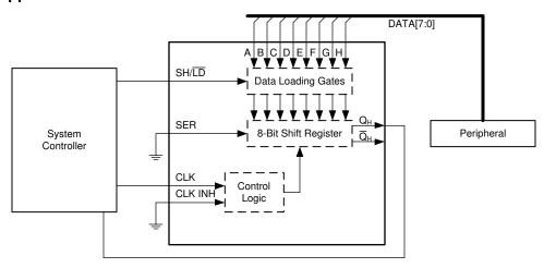
Figure 9-1. Input Expansion with Shift Registers
