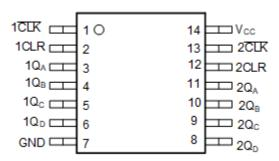
Figure 5-1. SN74LV393B-EP: PW Package, 14-Pin TSSOP (Top View)
