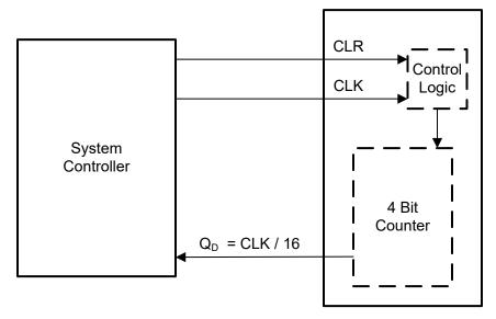
Figure 9-1. System Clock Divider
