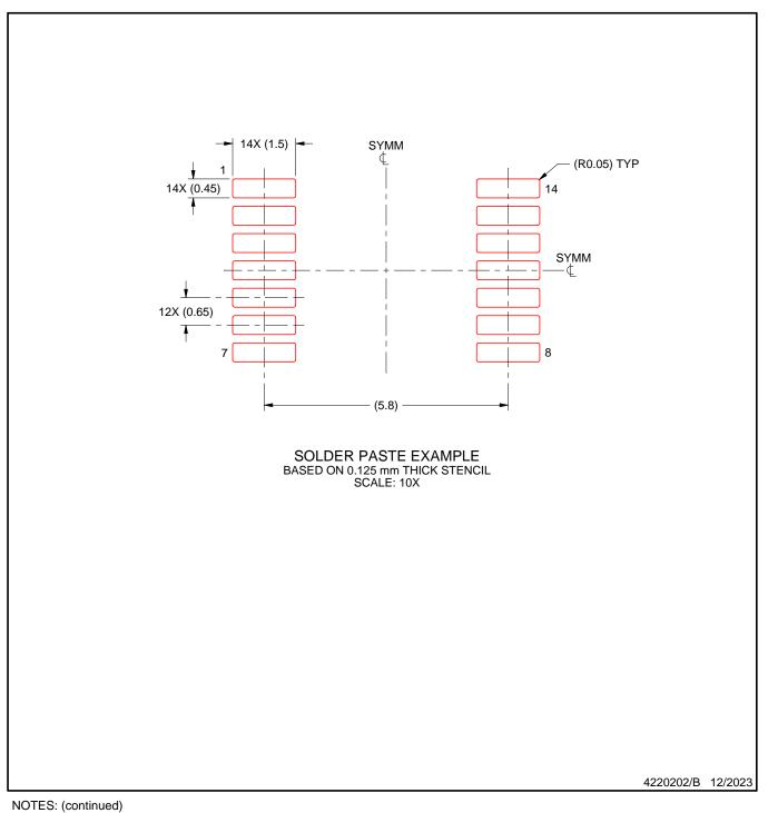
8. Laser cutting apertures with trapezoidal walls and rounded corners may offer better paste release. IPC-7525 may have alternate design recommendations.
