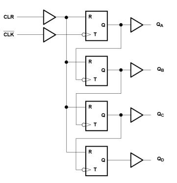
Logic Diagram (Positive Logic)
