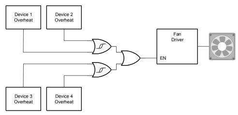
Figure 8-1. Typical Application Block Diagram
