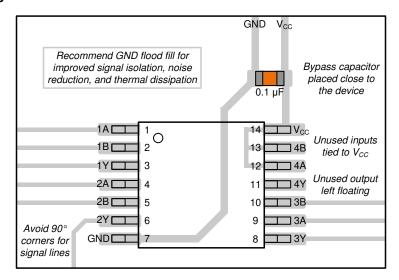
Figure 8-3. Example Layout for the SN74LV4T32-EP
