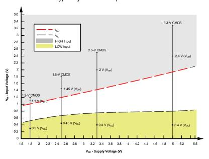
Figure 7-2. LVxT Input Voltage Levels
