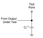
(1) C<sub>L</sub> includes probe and test-fixture capacitance.
