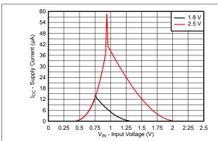
Figure 5-1. Supply Current Across Input Voltage 1.8-V and 2.5-V | Figure 5-2. Supply Current Across Input Voltage 3.3-V and 5.0-V
