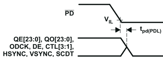
Figure 8-7. Delay From \overline{PD} Low to Hi-Z Outputs
