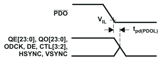
Figure 8-8. Delay From \overline{PDO} Low to Hi-Z Outputs
