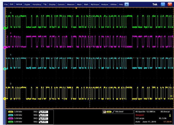
THVD2410 V_{CC} = 3.3\text{ V} R_L = 50\ \Omega Random (PRBS7) data at 500 kbps
