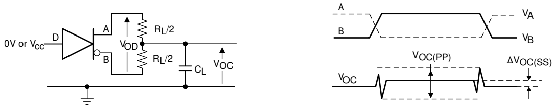
Figure 6-2. Measurement of Driver Differential and Common-Mode Output With RS-485 Load
