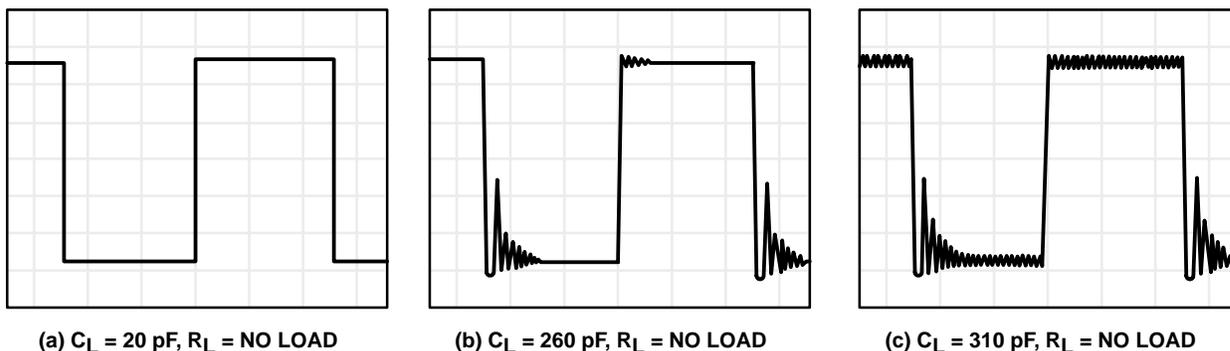
**Figure 112. Effect of Capacitive Loads in Low-Bias Mode**
