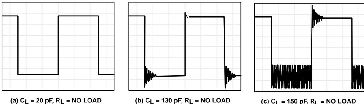
**Figure 110. Effect of Capacitive Loads in High-Bias Mode**
