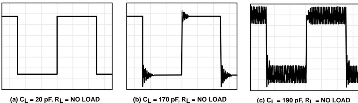
**Figure 111. Effect of Capacitive Loads in Medium-Bias Mode**
