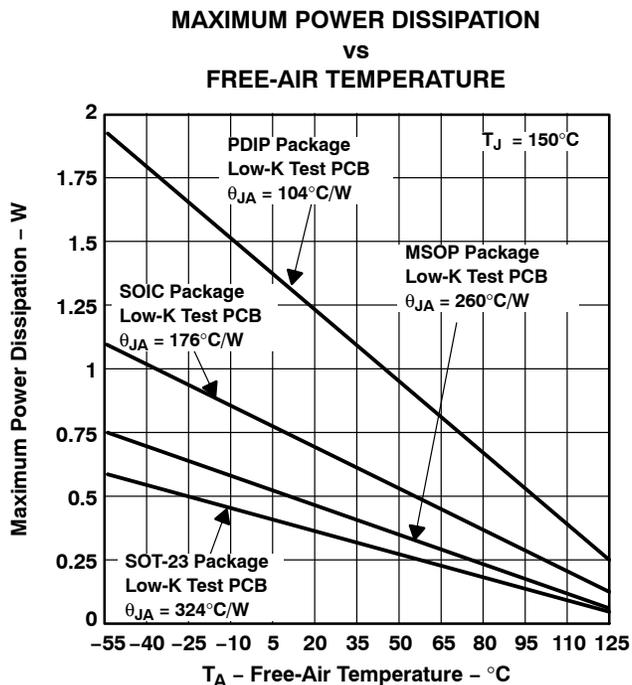
NOTE A: Results are with no air flow and using JEDEC Standard Low-K test PCB.
