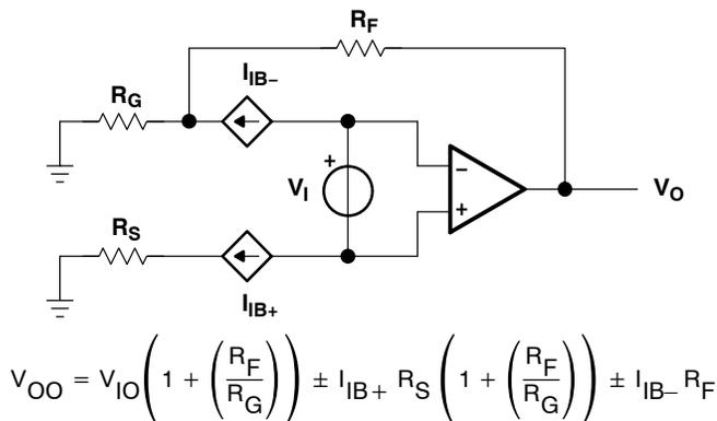
**Figure 32. Output Offset Voltage Model**
