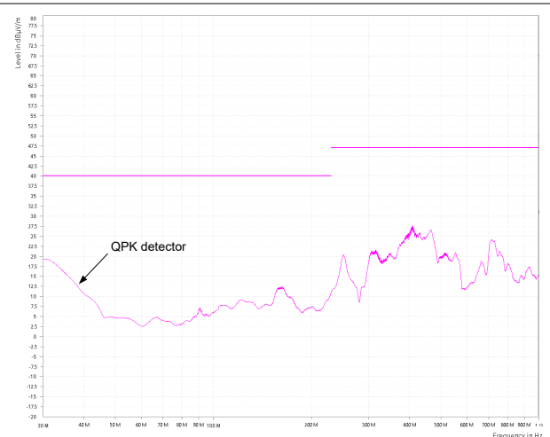
Figure 9-11. CISPR 32 Class B Radiated Emissions: Vertical Polarization
