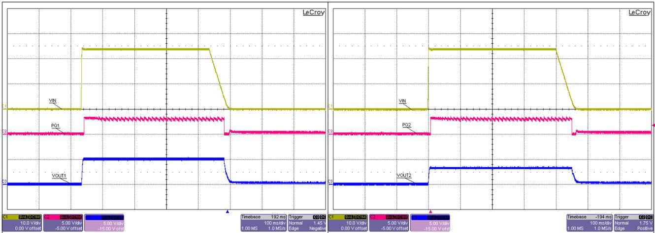
Figure 8-6. Start-up and Shutdown, VOUT1 = 5V
