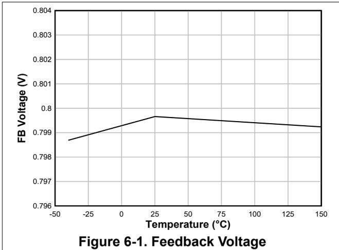
**Figure 6-1. Feedback Voltage**
