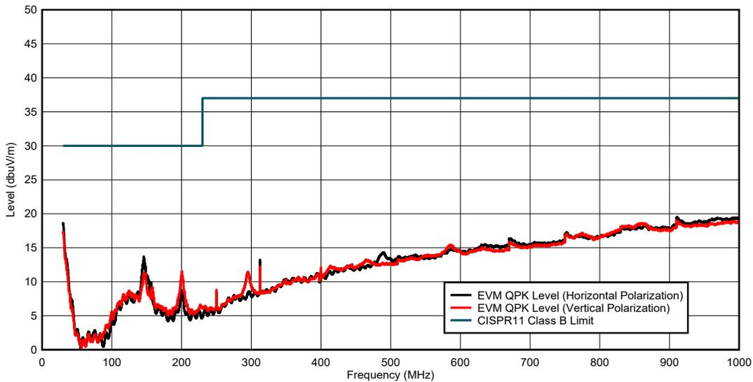
$V_{OUT} = 5V, V_{OUT2} = 3.3V, I_{OUT1} = 3A, I_{OUT2} = 3A, F_{SW} = 1MHz$
