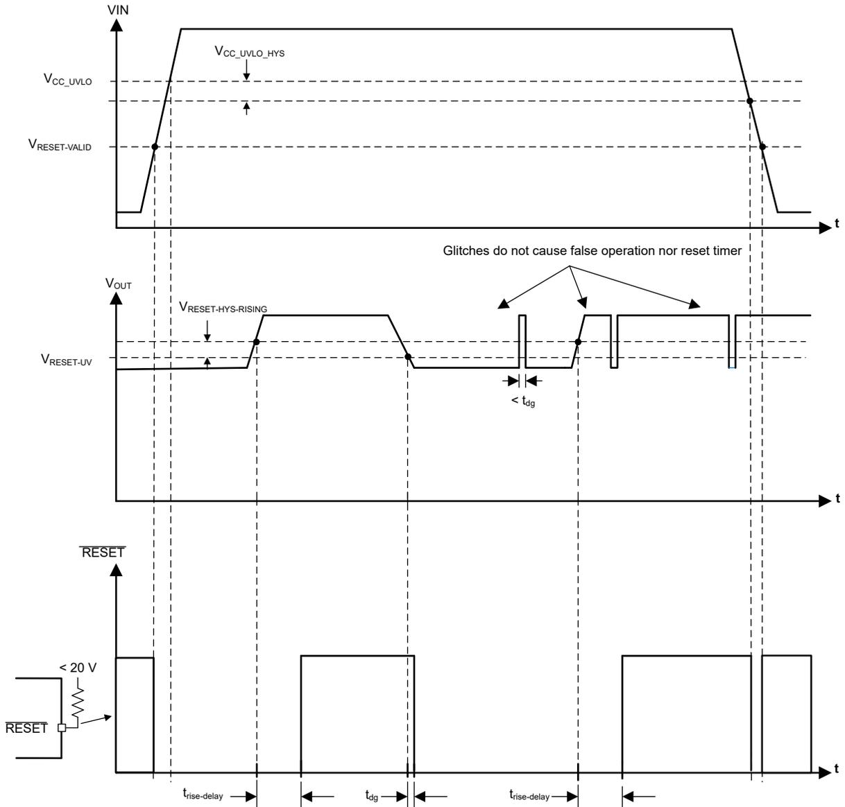
**Figure 7-6. PG Timing Diagram (Excludes OV Events)**
