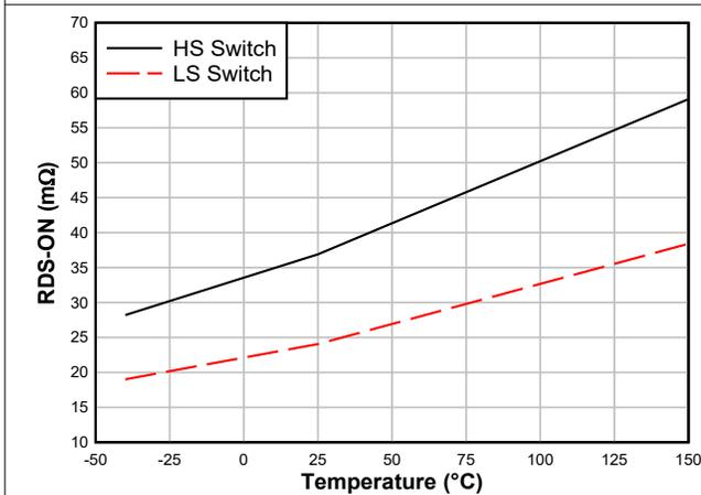
**Figure 6-3. High-side and Low-side Switches**
