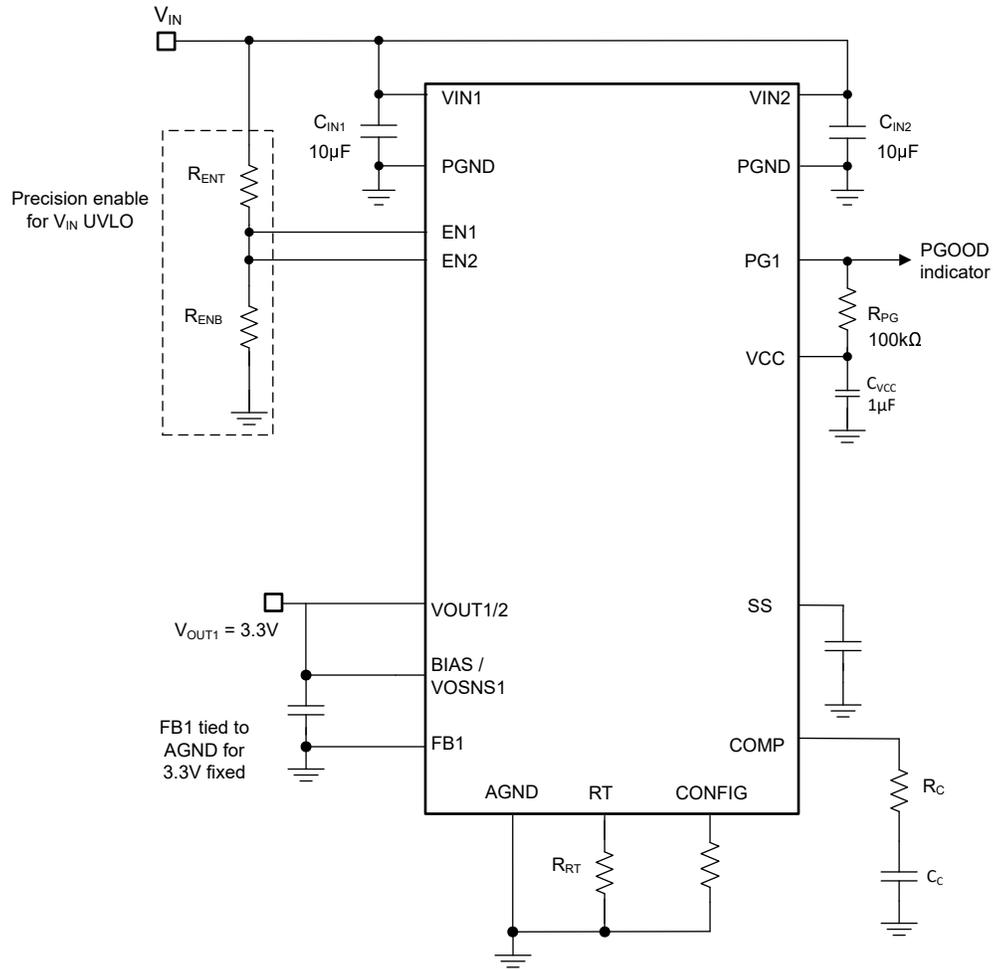
**Figure 7-3. High-efficiency, Single Output 2-Phase Step-Down Converter**
