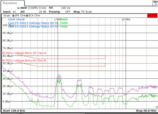
$V_{OUT1} = 5V, V_{OUT2} = 3.3V, I_{OUT1} = 3A, I_{OUT2} = 3A, F_{SW} = 1MHz$
