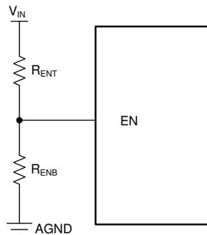
**Figure 7-2. VIN UVLO Using the EN Pin**
