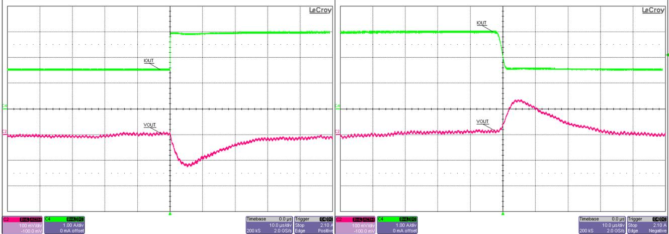
VOUT1 = 5V, IOUT1 = 3A to 6A at 1A/μs
