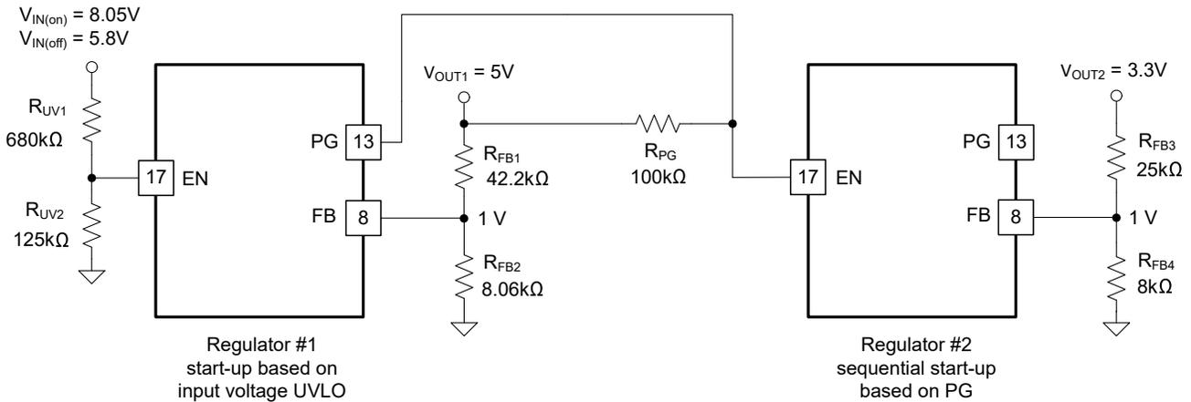
**Figure 7-8. TLVM1440x Sequencing Implementation Using PG and EN|**
