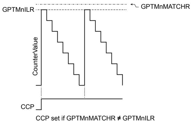
Figure 10-7 on page 652 shows how the CCP output operates when the **PLO** and **MRSU** bits are set and the **GPTMTnMATCHHR** value is the same as the **GPTMTnILR** value. In this situation, if the **PLO** bit is 0, the CCP signal goes high when the **GPTMTnILR** value is loaded and the match would be essentially ignored.
