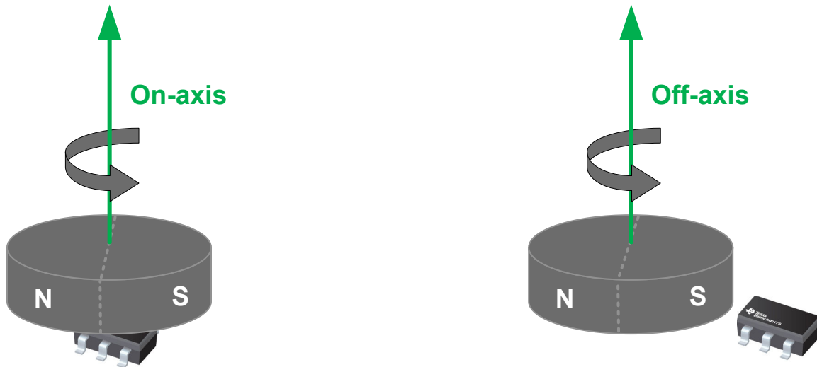
Figure 8-16. On-Axis vs. Off-Axis Angle Measurements
