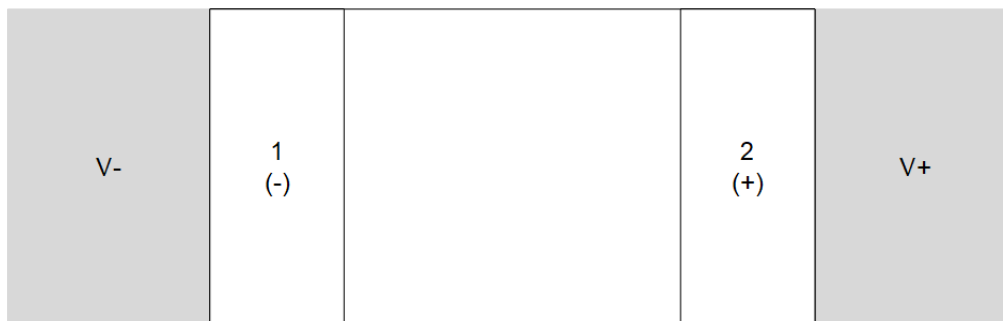
Figure 10-1. DEC Package Recommended Layout
