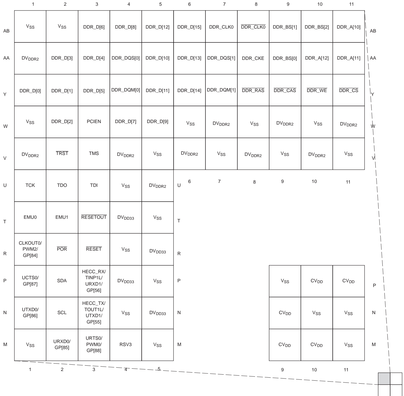
Figure 2-6. ZDU Pin Map [Quadrant A]
