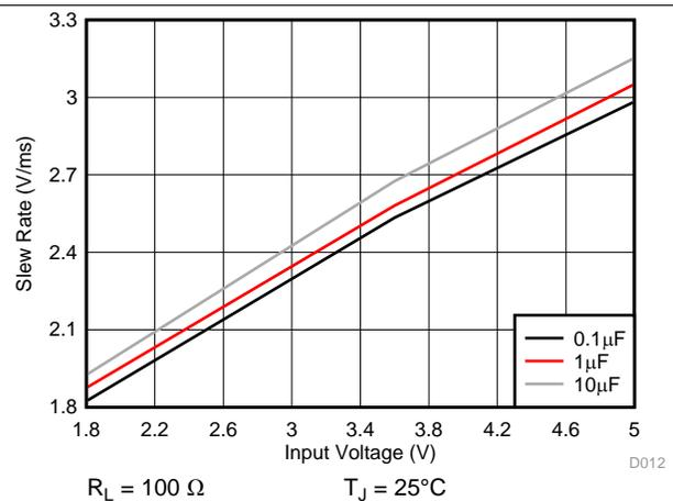
Figure 12. Slew Rate vs Input Voltage Across Load Capacitance
