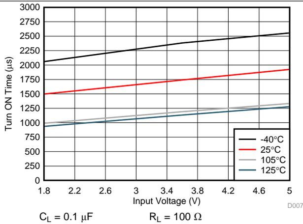
Figure 7. Turn ON Time vs Input Voltage
