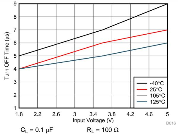
Figure 16. Turn OFF Time vs Input Voltage
