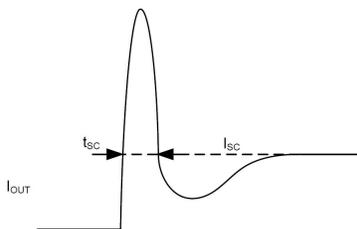
Figure 29. Output Short Circuit Response
