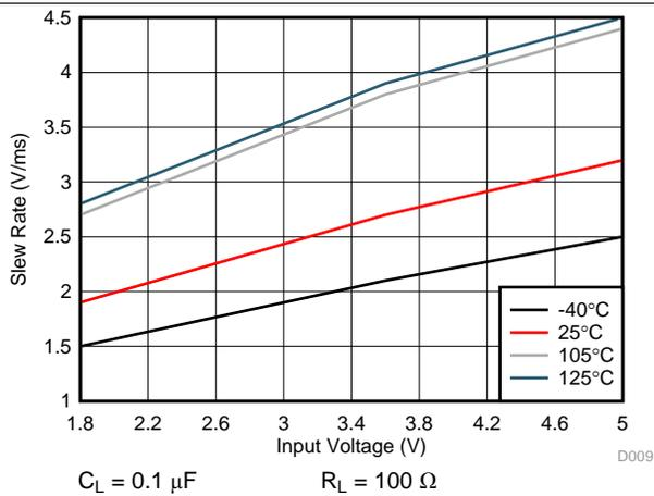
Figure 9. Output Slew Rate vs Input Voltage
