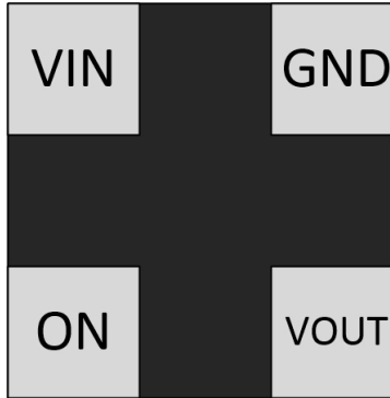
Figure 5-1. TPS22991 RAA Package, 4-Pin UQFN (Top View)
