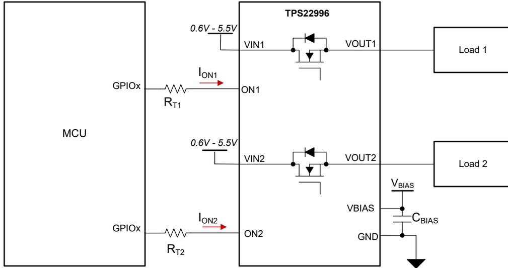
**Figure 8-1. TPS22996 Adjustable Rise Time Configuration**
