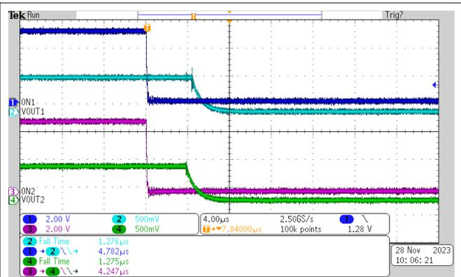
$V_{BIAS} = 5 \text{ V}$        $V_{IN} = 0.6 \text{ V}$        $I_{ON} = 20 \mu\text{A}$
