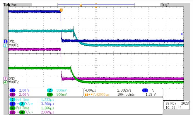
$V_{BIAS} = 5 \text{ V}$        $V_{IN} = 0.6 \text{ V}$        $I_{ON} = 100 \mu\text{A}$
