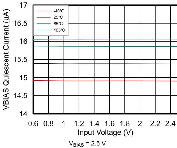
**Figure 6-3. V<sub>BIAS</sub> Quiescent Current vs Input Voltage Both Channels**
