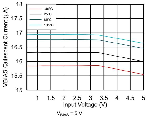
**Figure 6-4. V<sub>BIAS</sub> Quiescent Current vs Input Voltage Both Channels**
