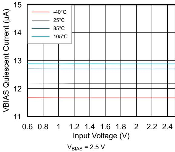
**Figure 6-1. V<sub>BIAS</sub> Quiescent Current vs Input Voltage Single Channel**
