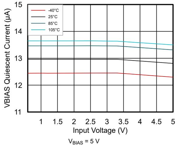
**Figure 6-2. V<sub>BIAS</sub> Quiescent Current vs Input Voltage Single Channel**
