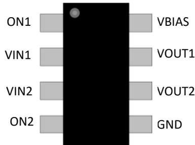
**Figure 5-1. DRL Package, 8-Pin SOT (Top View)**
