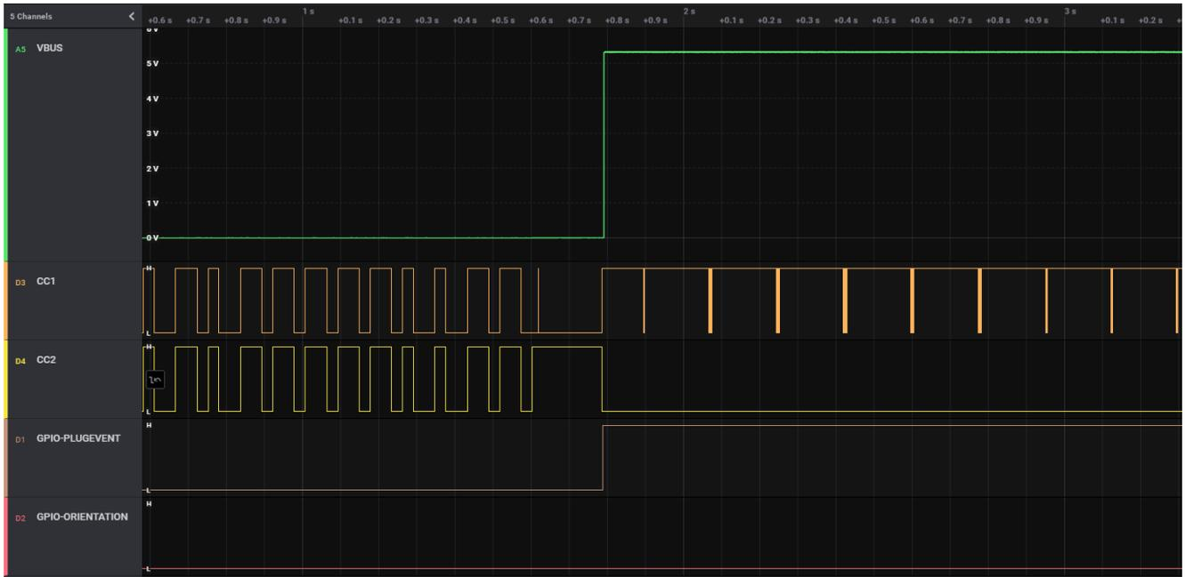
Figure 9-23. USB SuperSpeed Mux Control - Normal Orientation
