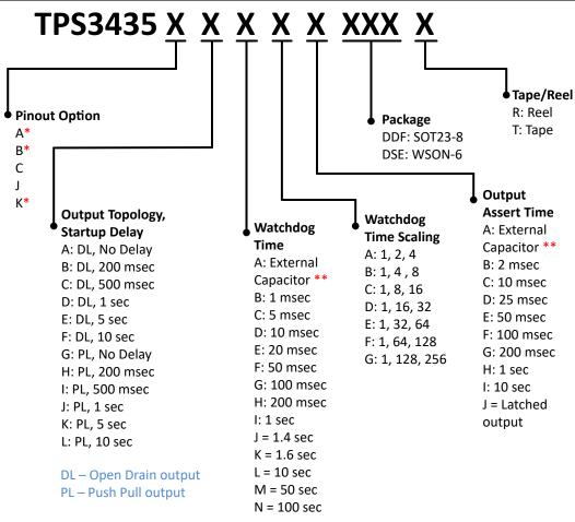
\* Pinout option supports Start up Delay settings of "No Delay" and "10 sec" only. \*\* Capacitor programmable time feature available with pinout options A, B & K. For fixed time and latched output features use pinout options C & J. Refer 'Mechanical, Packaging and Orderable Information' section for list of released orderable. For any other orderable, contact local TI support.
