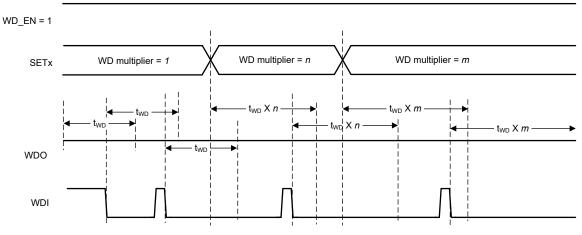
Figure 7-9. Watchdog Behavior with SETx Pin Status
