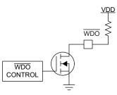
Figure 8-2. Open-Drain WDO Configuration
