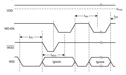
Figure 7-7. Watchdog Enable: WD-EN Pin Control
