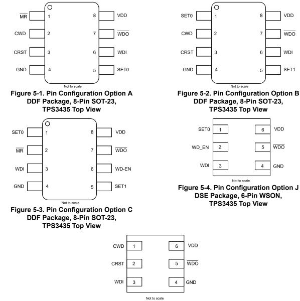
Figure 5-5. Pin Configuration Option K DSE Package, 6-Pin WSON, **TPS3435** Top View
