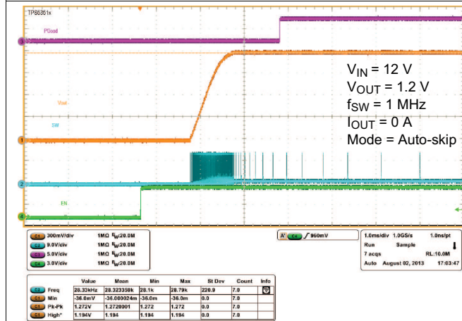
Figure 19. Auto-Skip Mode Load Transient
