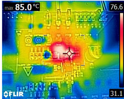
Figure 5-7. Thermal Image – 5V Output, TPS54KB20EVM, 6 Layers
