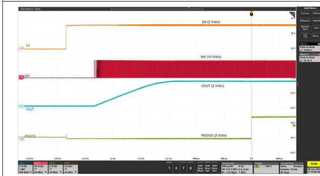
V_{IN} = 12V V_{OUT} = 3.3V I_{OUT} = 25A Figure 7-10. Start-Up With EN
