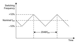
Figure 8-11. Spread Spectrum Clocking Behavior
