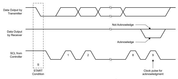
Figure 8-17. Acknowledge on the I<sup>2</sup>C Bus
