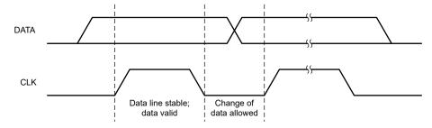
Figure 8-16. Bit Transfer on the Serial Interface
