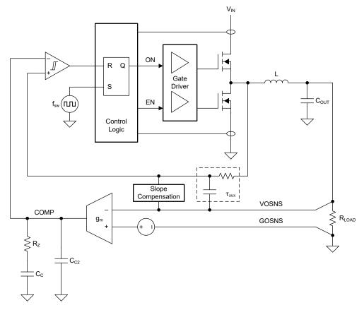
Figure 8-1. Fixed-Frequency DCS Control Topology (Simplified)
