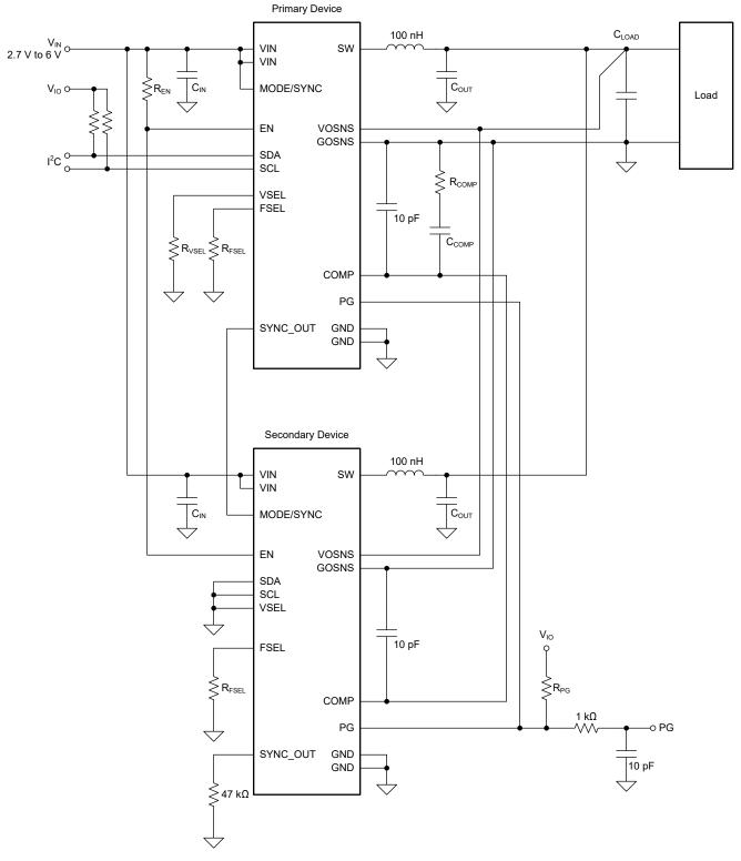
Figure 8-14. Two TPS6287x-Q1 Devices in a Stacked Configuration
