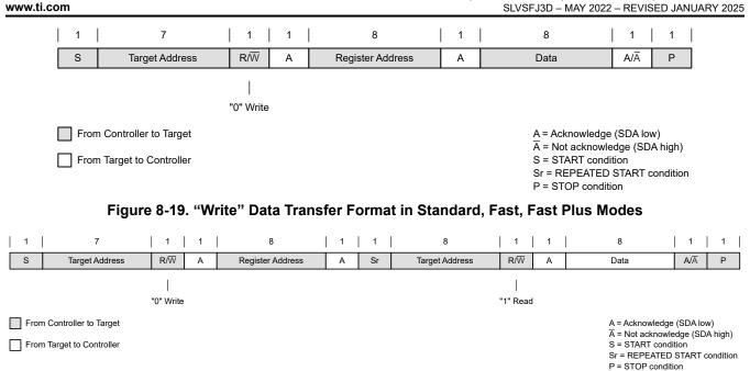
Figure 8-20. "Read" Data Transfer Format in Standard, Fast, Fast Plus Modes
