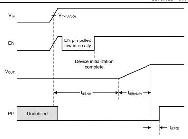
Figure 8-7. Start-Up Timing When EN is Pulled Up to VIN
