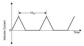
Figure 8-3. Discontinuous Conduction Mode (PWM-DCM) Current Waveform
