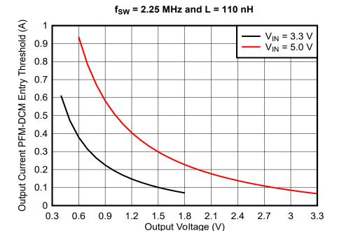
Figure 8-5. Output Current PFM-DCM Entry Threshold
