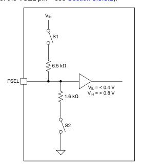
Figure 8-10. FSEL R2D Converter Functional Block Diagram
