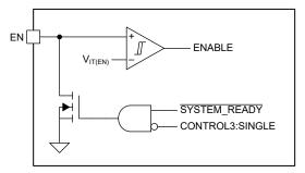
Figure 8-6. Enable Functional Block Diagram
