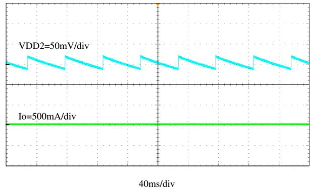
**Figure 8-10. VDD2 Output Voltage Ripple,  $I_{OUT} = 0\text{ A}$**
