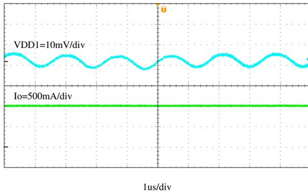
**Figure 8-13. VDD1 Output Voltage Ripple,  $I_{OUT} = 1\text{ A}$**
