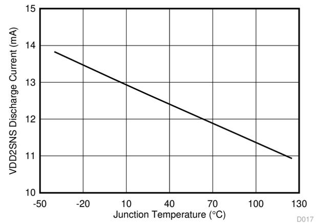
**Figure 6-17. VDD2SNS Discharge Current vs Junction Temperature**
