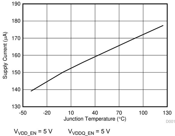
**Figure 6-1. VCC\_5V Supply Current vs Junction Temperature**
