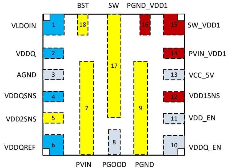
**Figure 5-1. 18-Pin VQFN RJE Package (Top View)**
