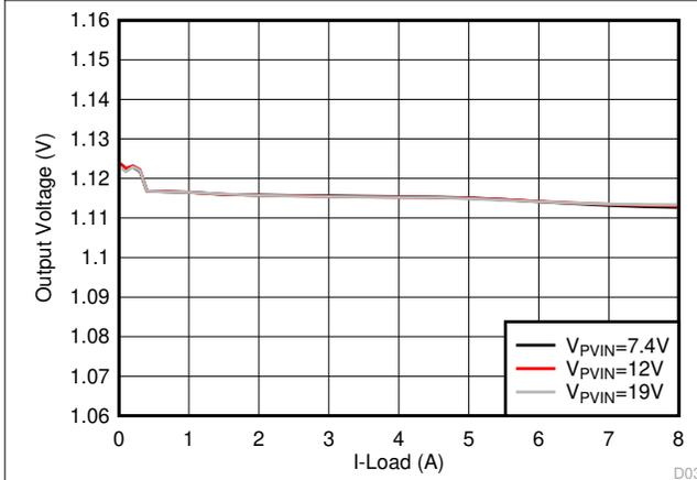
**Figure 8-5. VDD2 Load Regulation,  $V_{OUT} = 1.1\text{ V}$**
