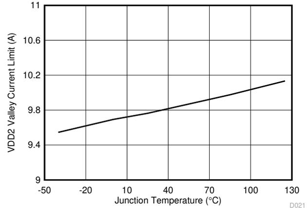
**Figure 6-20. VDD2 Valley Current Limit vs Junction Temperature**
