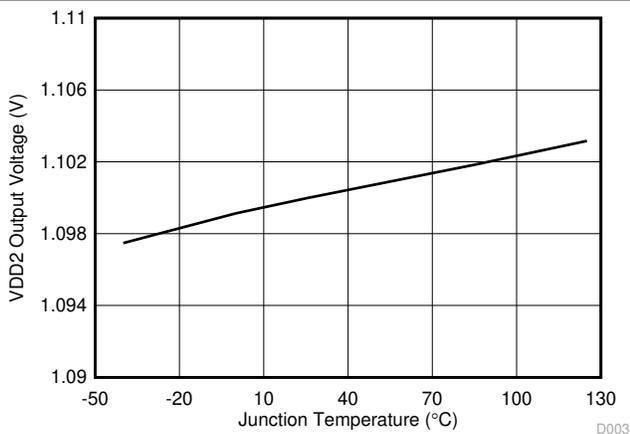
**Figure 6-3. VDD2 Output Voltage vs Junction Temperature**
