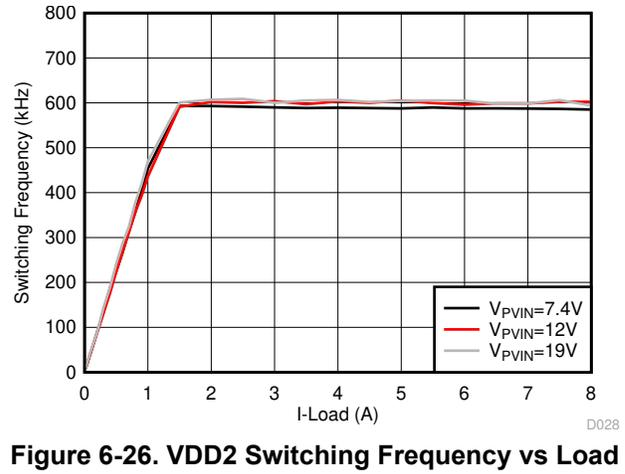
**Figure 6-26. VDD2 Switching Frequency vs Load Current**
