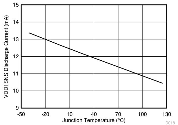
**Figure 6-18. VDD1SNS Discharge Current vs Junction Temperature**
