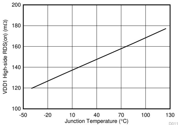
**Figure 6-11. VDD1 High-Side R\_DS(on) vs Junction Temperature**
