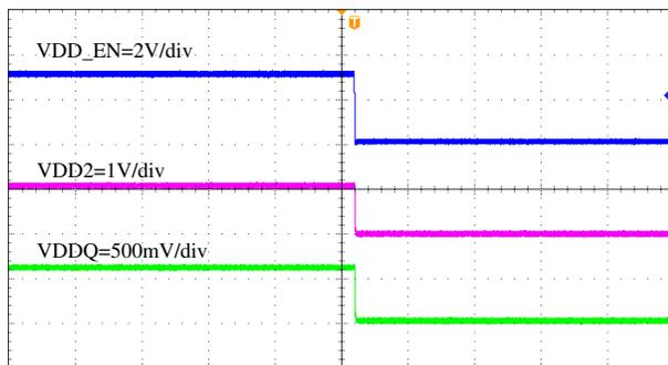
Figure 8-25. VDDQ Shutdown Through VDD\_EN
