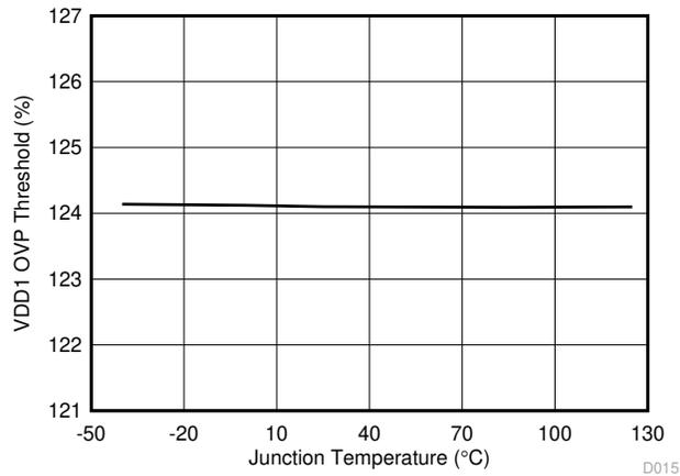
**Figure 6-15. VDD1 OVP Threshold vs Junction Temperature**
