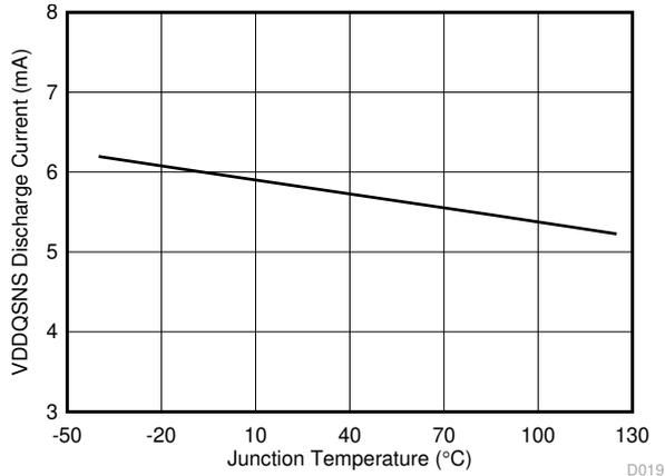
**Figure 6-19. VDDQSNS Discharge Current vs Junction Temperature**
