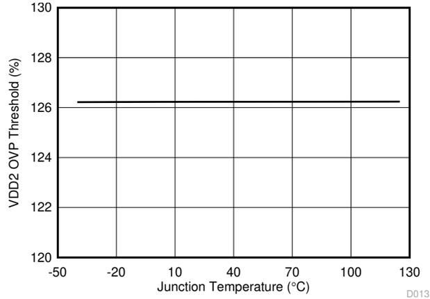
**Figure 6-13. VDD2 OVP Threshold vs Junction Temperature**
