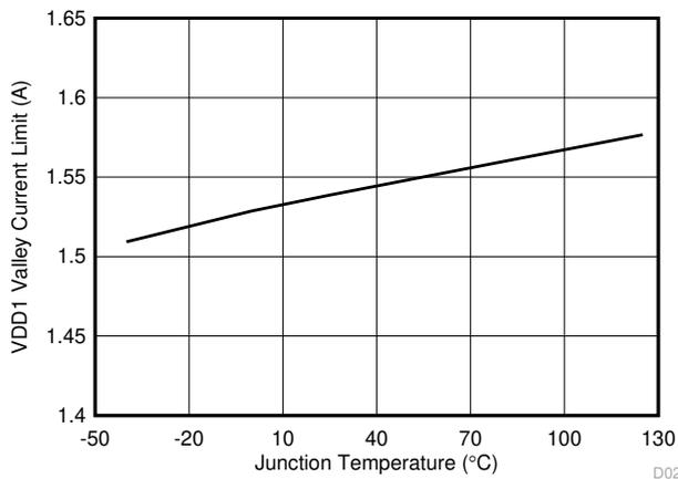
**Figure 6-21. VDD1 Valley Current Limit vs Junction Temperature**
