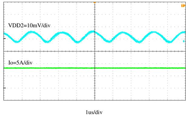
**Figure 8-12. VDD2 Output Voltage Ripple,  $I_{OUT} = 8\text{ A}$**
