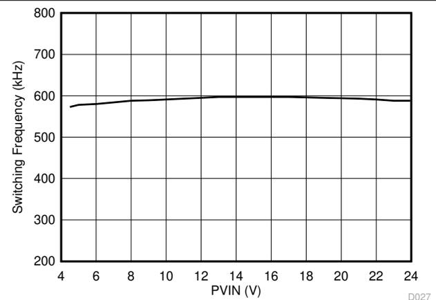
**Figure 6-24. VDD2 Switching Frequency vs Input Voltage**
