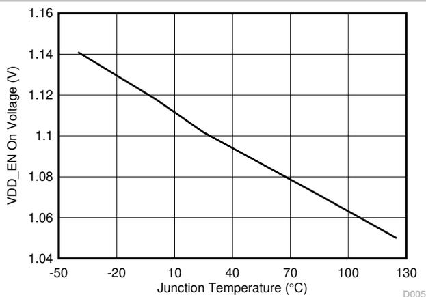
**Figure 6-5. Enable On Voltage (VDD\_EN) vs Junction Temperature**
