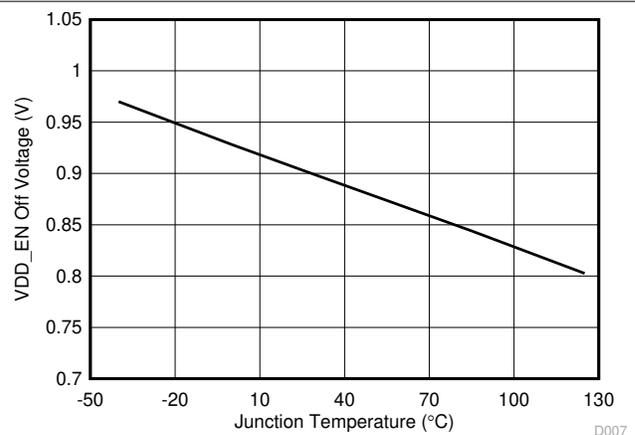
**Figure 6-6. Enable Off Voltage (VDD\_EN) vs Junction Temperature**
