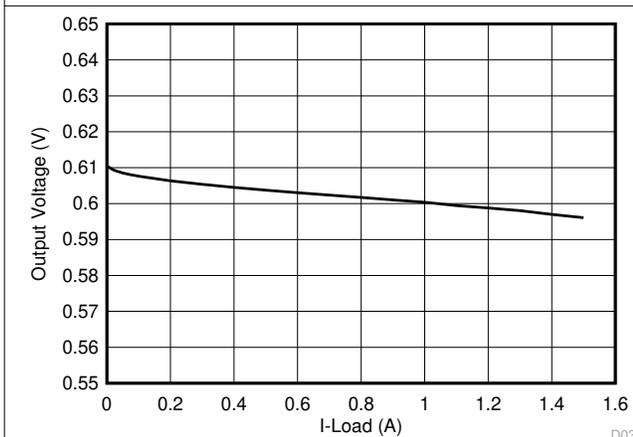
**Figure 8-7. VDDQ Load Regulation,  $V_{OUT} = 0.6\text{ V}$**
