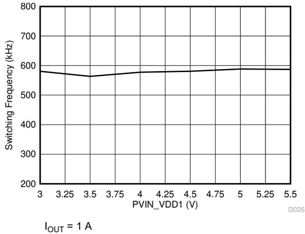
**Figure 6-25. VDD1 Switching Frequency vs Input Voltage**
