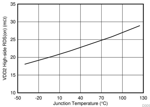
**Figure 6-9. VDD2 High-Side R\_DS(on) vs Junction Temperature**
