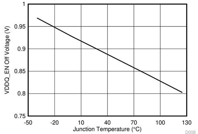
**Figure 6-8. Enable Off Voltage (VDDQ\_EN) vs Junction Temperature**
