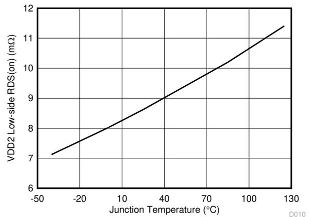
**Figure 6-10. VDD2 Low-Side R\_DS(on) vs Junction Temperature**
