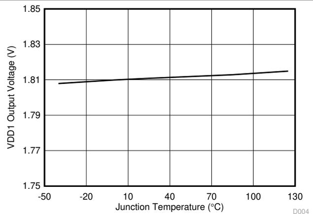
**Figure 6-4. VDD1 Output Voltage vs Junction Temperature**
