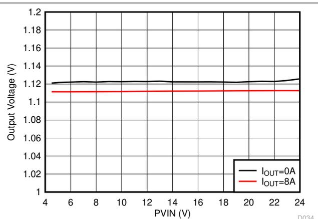
**Figure 8-8. VDD2 Line Regulation,  $V_{OUT} = 1.1\text{ V}$**
