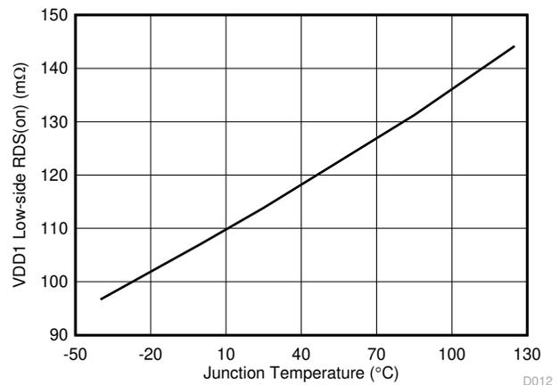
**Figure 6-12. VDD1 Low-Side R\_DS(on) vs Junction Temperature**
