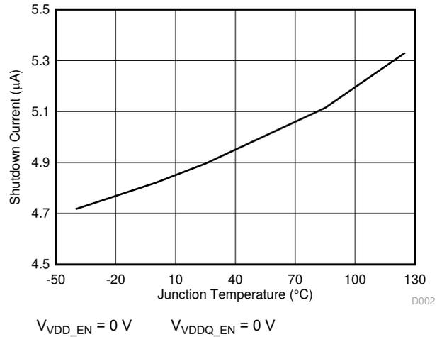
**Figure 6-2. VCC\_5V Shutdown Current vs Junction Temperature**
