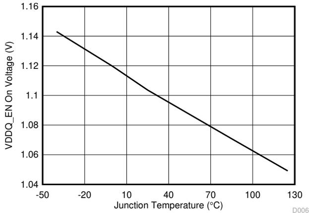
**Figure 6-7. Enable On Voltage (VDDQ\_EN) vs Junction Temperature**
