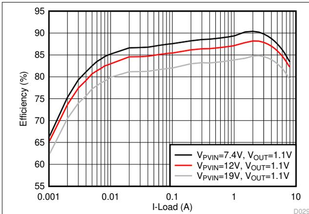
**Figure 8-3. VDD2 Efficiency Curve,  $V_{OUT} = 1.1\text{ V}$**
