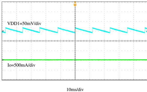
**Figure 8-11. VDD1 Output Voltage Ripple,  $I_{OUT} = 0\text{ A}$**
