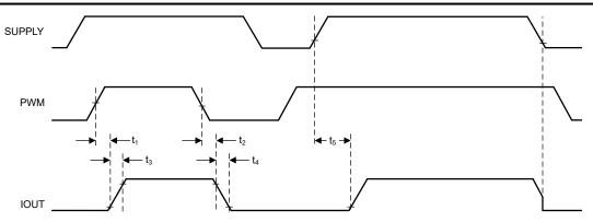
Figure 7-1. Power-On Sequence and PWM Dimming Timing
