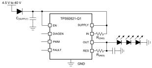
Figure 3-1. Typical Application Diagram
