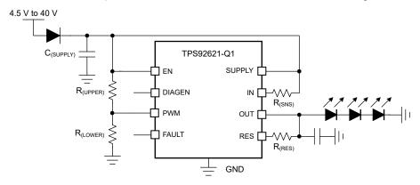
Figure 7-2. Application Schematic for Supply Control LED Brightness
