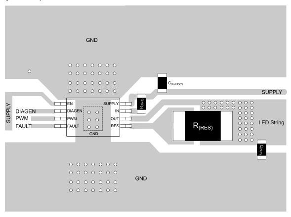
Figure 8-7. TPS92621-Q1 Example Layout Diagram
