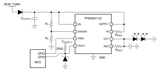
Figure 8-4. Typical Application Schematic
