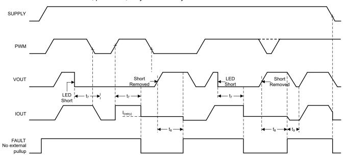
Figure 7-3. LED Short-to-GND Detection and Recovery Timing Diagram
