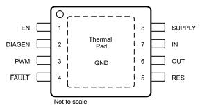
Figure 5-1. DGN Package 8-Pin HVSSOP With PowerPAD™ Integrated Circuit Package (Top View)
