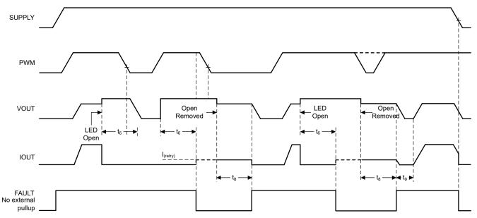
Figure 7-4. LED Open-Circuit Detection and Recovery Timing Diagram
