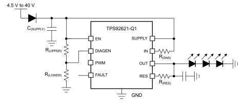
Figure 7-5. Application Schematic For DIAGEN
