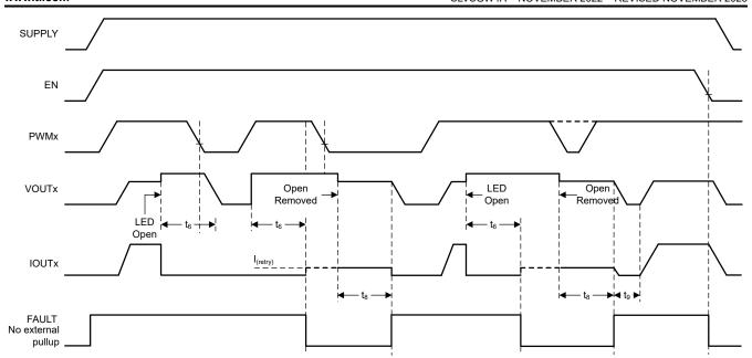
Figure 6-4. LED Open-Circuit Detection and Recovery Timing Diagram
