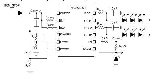
Figure 7-1. Typical Application Schematic
