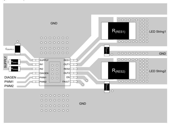
Figure 7-7. TPS92622-Q1 Example Layout Diagram
