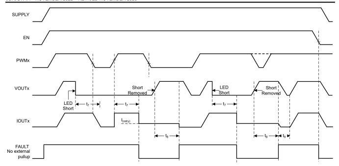
Figure 6-3. LED Short-to-GND Detection and Recovery Timing Diagram
