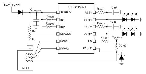
Figure 7-4. Typical Application Schematic
