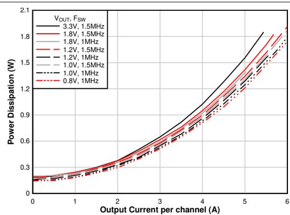
Figure 6-9. Power Dissipation vs Output Current
