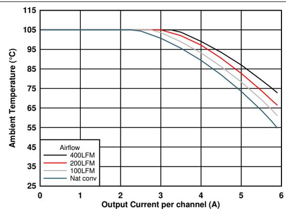
$F_{sw} = 2.0\text{ MHz}$  Dual 3.3-V outputs  $I_{OUT1} = I_{OUT2}$
