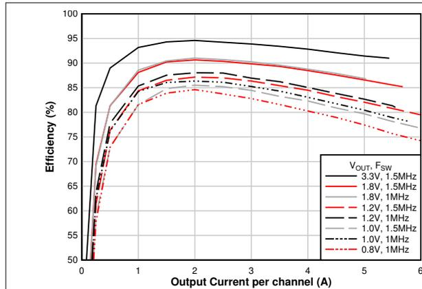
Figure 6-8. Efficiency vs Output Current
