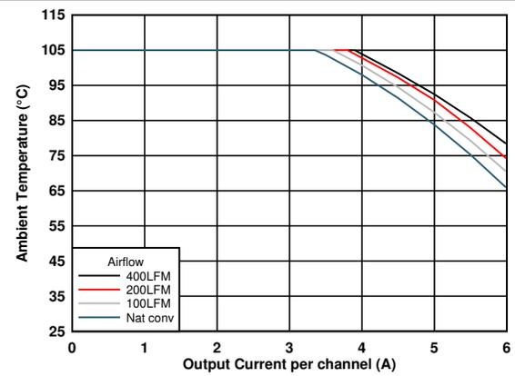
$F_{sw} = 1.0\text{ MHz}$  Dual 1.2-V outputs  $I_{OUT1} = I_{OUT2}$
