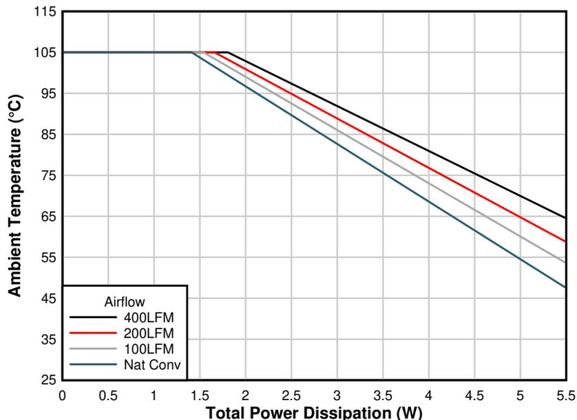
Figure 7-6. Ambient Temperature Versus Total Power Dissipation
