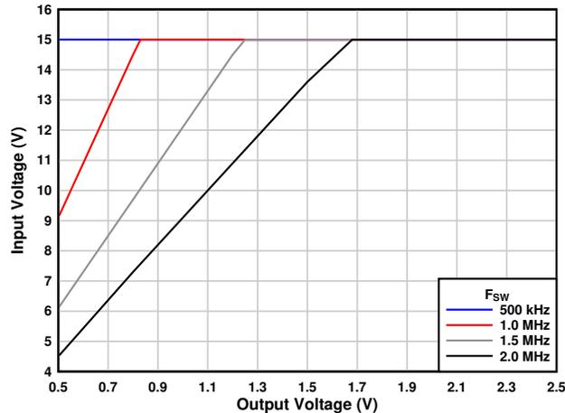
**Figure 7-3. Maximum Input Voltage**
