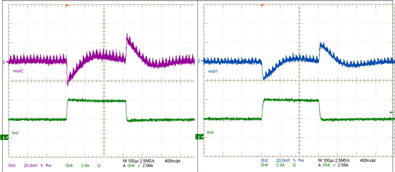
**Figure 8-4. Transient Response  $V_{OUT2}$**
