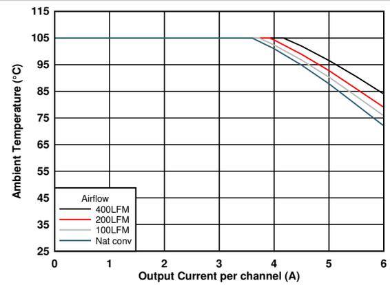
$F_{SW} = 1.0\text{ MHz}$  Dual 0.8-V outputs  $I_{OUT1} = I_{OUT2}$
