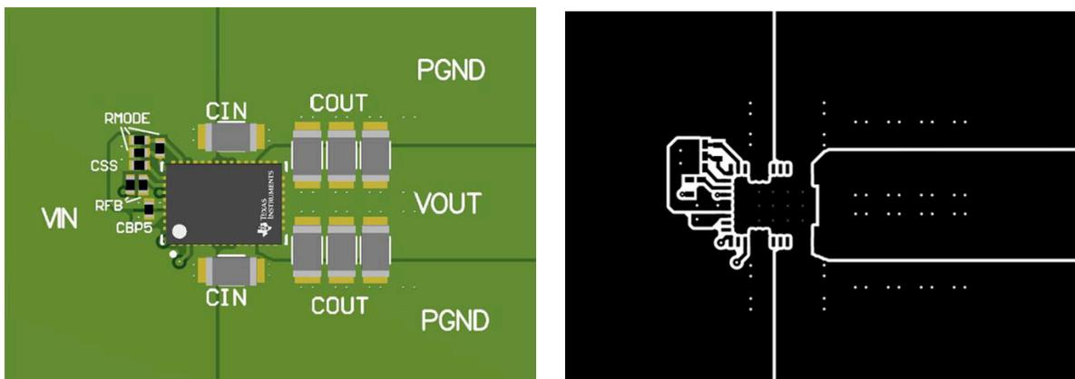
Figure 10-2. Typical Parallel-Output Layout
