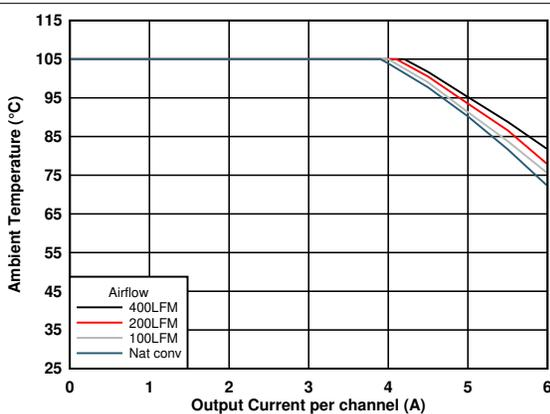
$F_{SW} = 1.5\text{ MHz}$  Dual 1.2-V outputs  $I_{OUT1} = I_{OUT2}$
