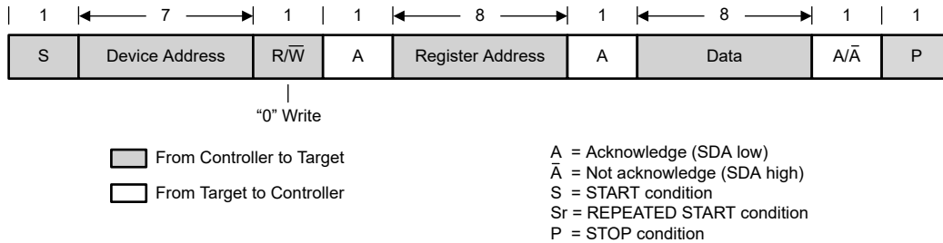
Figure 7-7. Write Data Transfer Format in Standard Modes, Fast Modes, and Fast-Plus Modes
